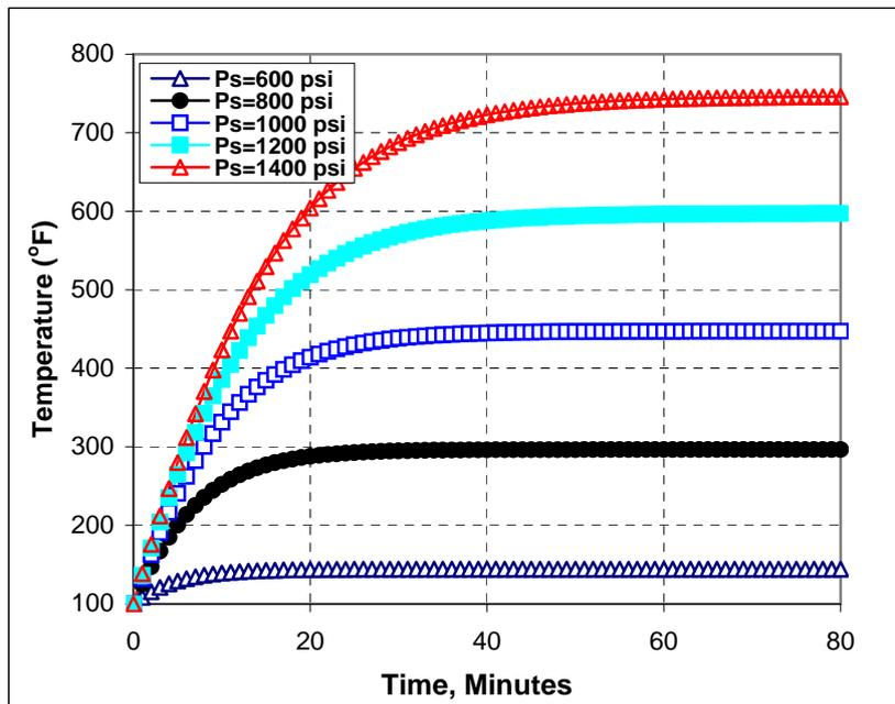
Figure 3 - Influence of surface pressure on bit temperature.
