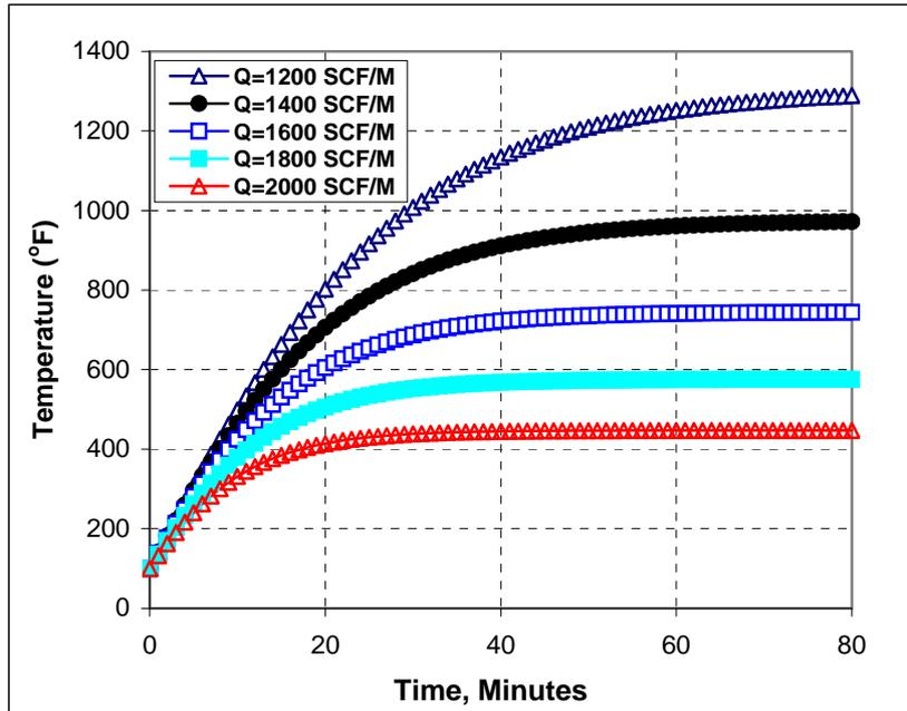
Figure 2 - Influence of flow rate on bottom hole bit temperature.
