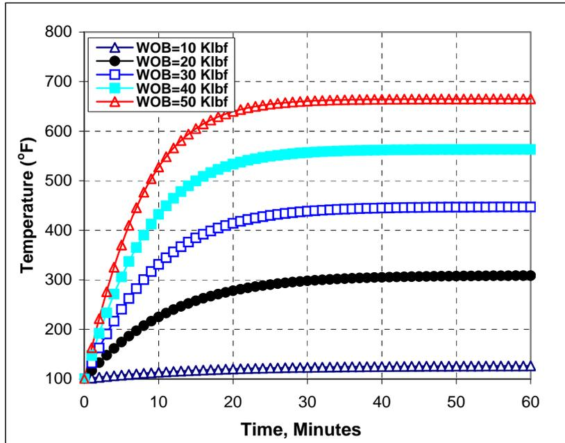
**Figure 6 - Effects of weight on bit on bit temperature (Q=2000 SCFM and n=50 rpm).**
