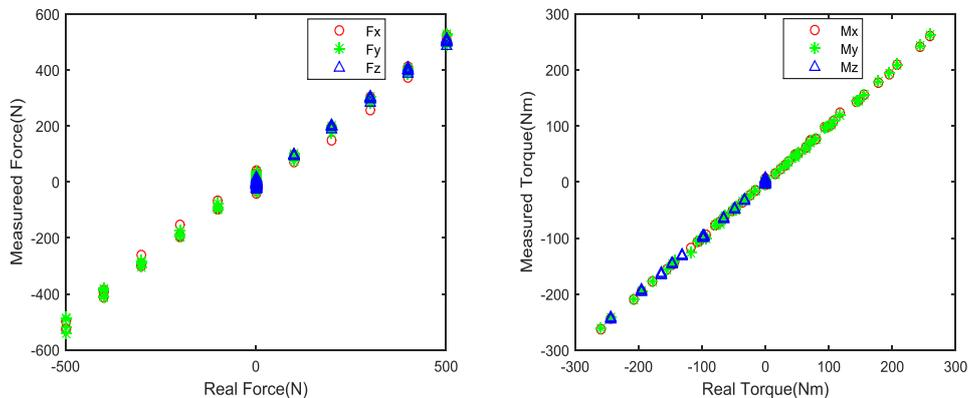
**Fig. 3** WFT calibration data plot
