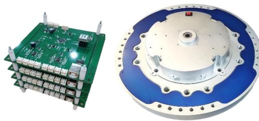
Fig. 6 Telemetry receiver and Transmitter
