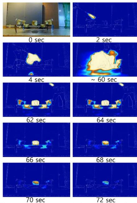
**Fig. 3** Thermal image of the fire-resistance test
