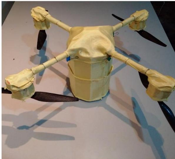
**Fig. 1** Aramid fiber-wrapped prototype of the developed robot system
