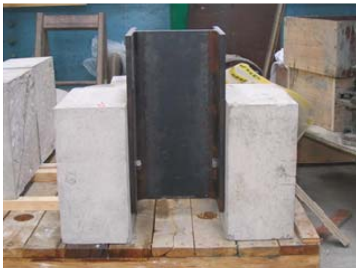
Fig. 2 Push off test specimen
