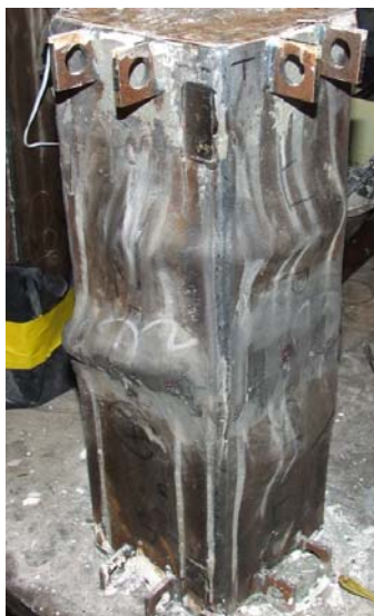
Fig. 12 Typical short column failure from test series
