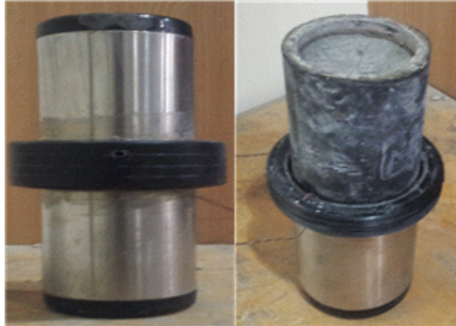
Fig. 2 Equipment for measuring temperature rise of concrete [1]
