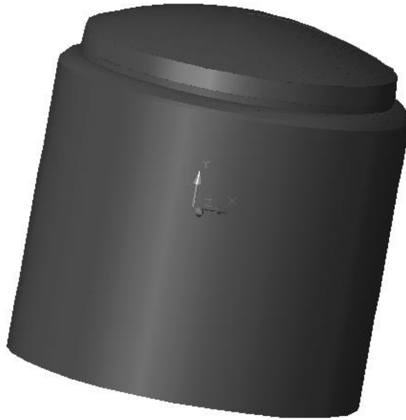
Fig. 16. - 3D Collapse Mechanism of the ASME vessel
