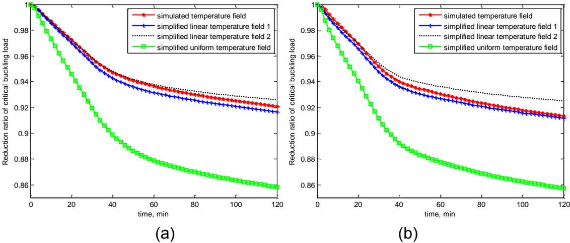
Fig. 3 Comparison of the reduction ratio,  $P_{cr,T}/P_{cr,20}$ , of a one side protected channel section. (a) 300x70x30x3; (b) 150x50x20x1.5
