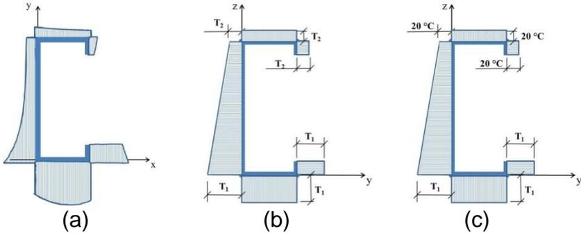
Fig. 2 Temperature fields. (a) simulated temperature field; (b) simplified linear temperature 1; (c) simplified linear temperature 2
