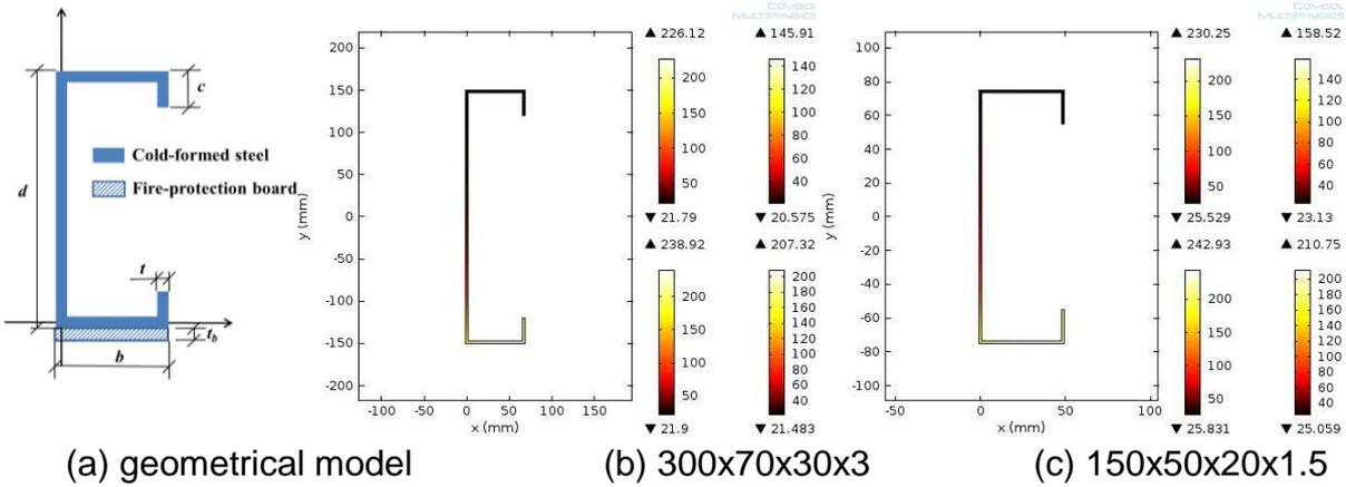
Fig. 1 Temperature distribution on the one-side protected cold-formed steel cross-sections
