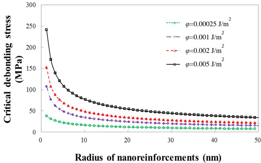
Figure 1. Effects of the interfacial adhesive energy ( $\phi$ ) on the critical debonding stress with an increased radius of SiO<sub>2</sub> nanoparticles.
