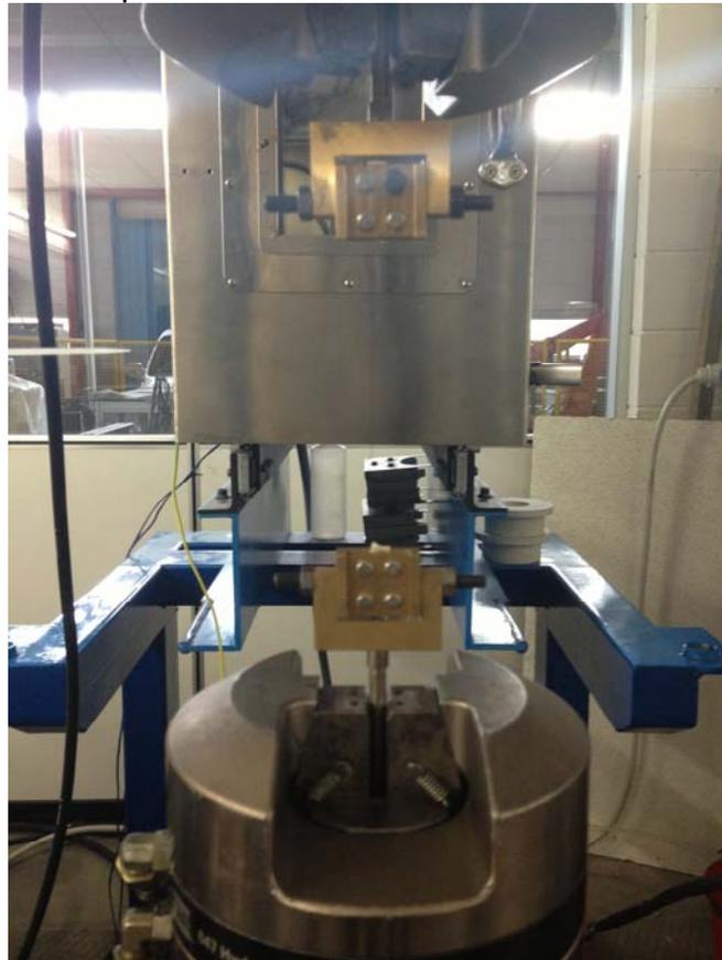
Fig. 1 Universal testing machine: detail of the additional devices used to fix the specimens to the grips.
