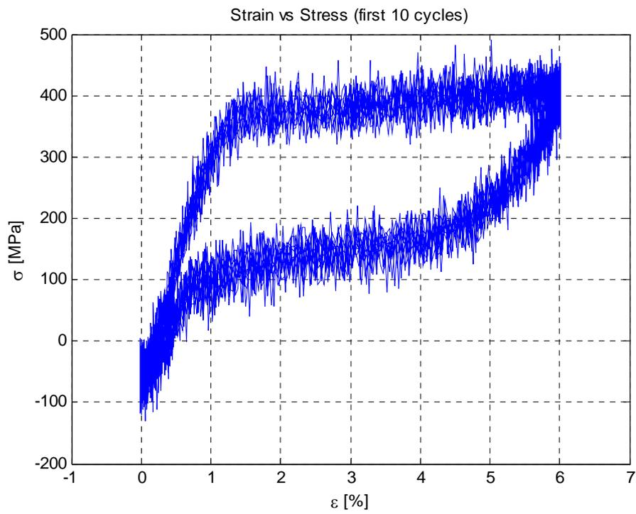
Fig. 4 Hysteresis cycles for material 2. Specimen length 50 mm. Training at 10%.
