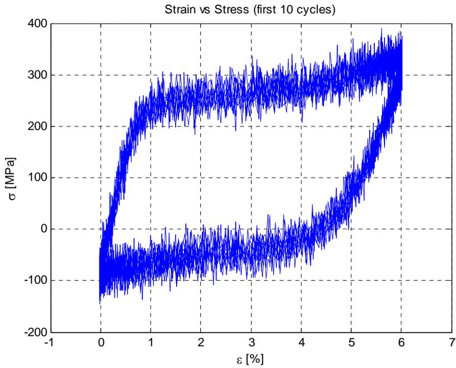
Fig. 3 Hysteresis cycles for material 1. Specimen length 100 mm. Training 8%.
