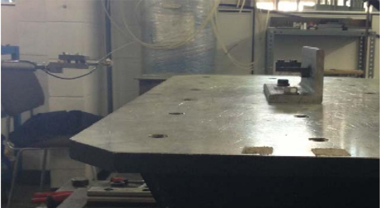
Fig. 2 Experimental mock-up adopted for testing wire specimens of length from 15 to 100 cm.
