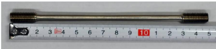
Fig. 1 Photograph of an SEA bar test specimen
