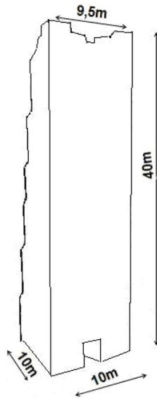
Fig. 3 Geometric characteristics of the minaret of Mansourah
