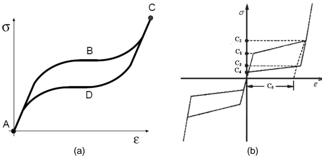
Fig. 12 (a) Typical and (b) idealization of the super-elasticity behavior of SMA
