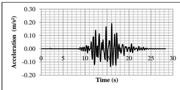
Fig. 11 Acceleration at node *A* situated at 40m under the simulated signal based on Ain Temouchent action (without SMA wires)
