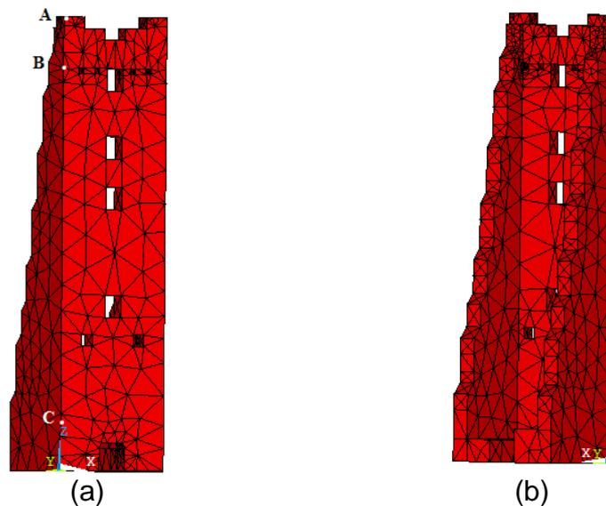
Fig. 5 Details of the 3D finite element model: (a) In front view, (b) Back view
