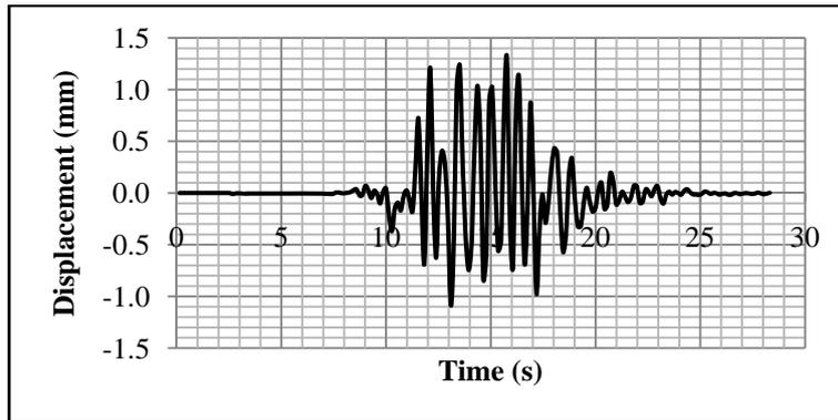
Fig. 15 Lateral displacement at node *A* situated at 40m under the simulated signal based on Ain-Temouchent action (with SMA wires)
