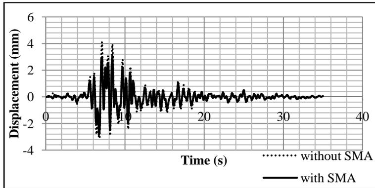
Fig. 17 Comparison of maximum displacement at node A under the 33% fraction of Boumerdes action with, and without the SMA wires
