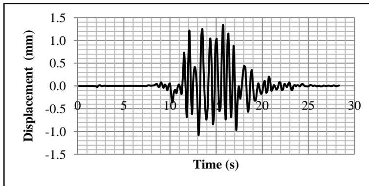
Fig. 10 Lateral displacement at node *A* situated at 40m under the simulated signal based on Ain-Temouchent action (without SMA wires)
