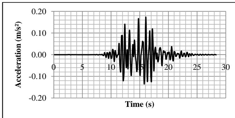
Fig. 16 Acceleration at node *A* situated at 40m under the simulated signal based on Ain-Temouchent (with SMA wires)
