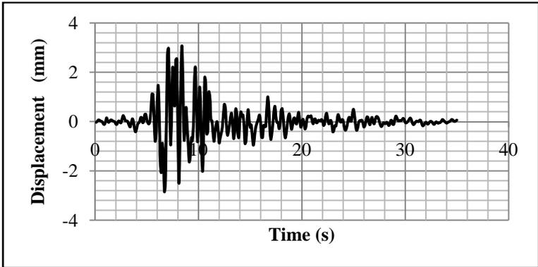
Fig. 13 Lateral displacement at node A situated at 40m under the 33% fraction of Boumerdes action (with SMA wires)
