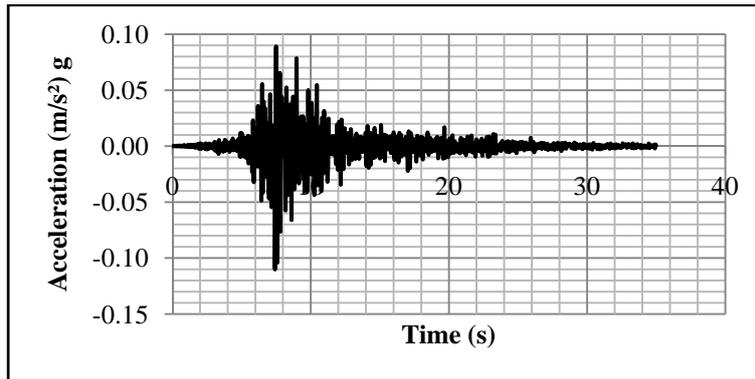
Fig. 6 Accelerogram record of the 33% fraction of Boumerdes earthquake (PGA=0.11g)
