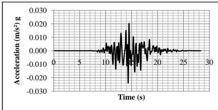
Fig. 7 Simulated signal from an aftershock of Ain-Temouchen earthquake (PGA=0.024g)
