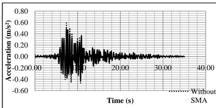
Fig. 18 Comparison of maximum acceleration at node A under the 33% fraction of Boumerdes action with, and without the SMA wires
