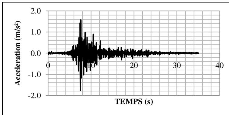
Fig. 9 Acceleration at node A situated at 40m under the 33% fraction of Boumerdes action (without SMA wires)
