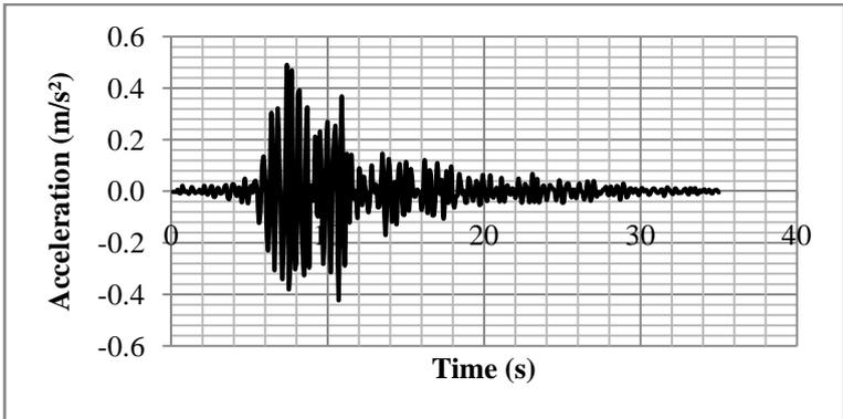
Fig. 14 Acceleration at node A situated at 40m under the 33% fraction of Boumerdes action (with SMA wires)
