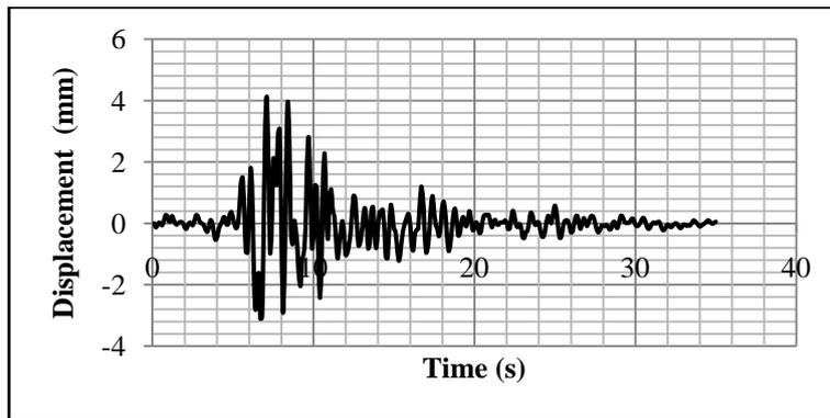
Fig. 8 Lateral displacement at node A situated at 40m under the 33% fraction of Boumerdes action (without SMA wires)
