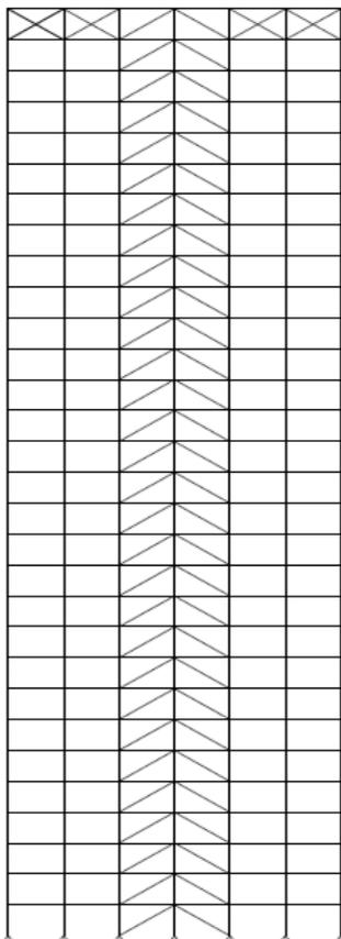
Figure 2. 30 Story V-bracing model
