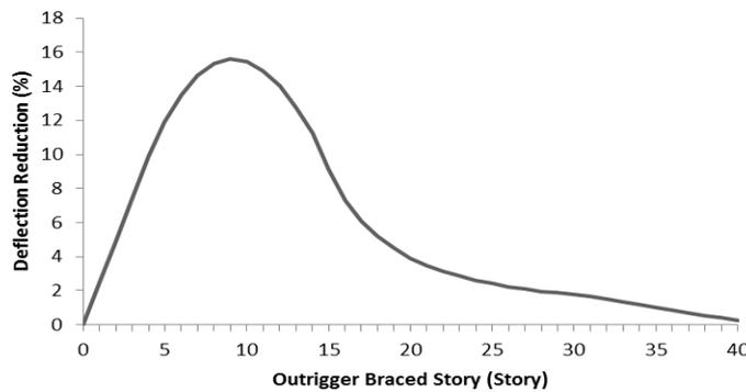
Figure 10. Deflection reduction for 40 story model (X-bracing core)
