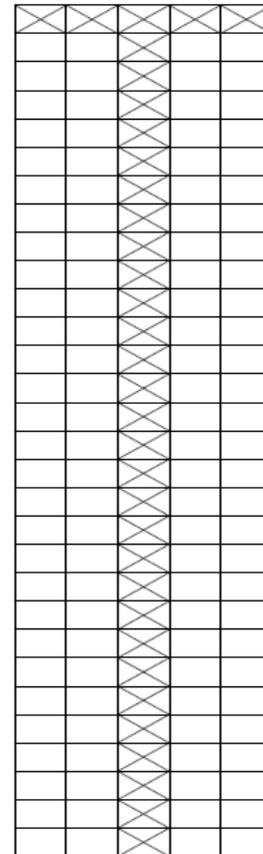
Figure 3. 30 Story X-bracing model
