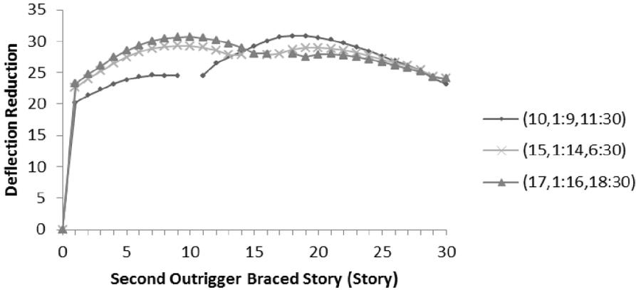
Figure 5. Deflection reduction caused by second outrigger for 30 story model (V-bracing core)
