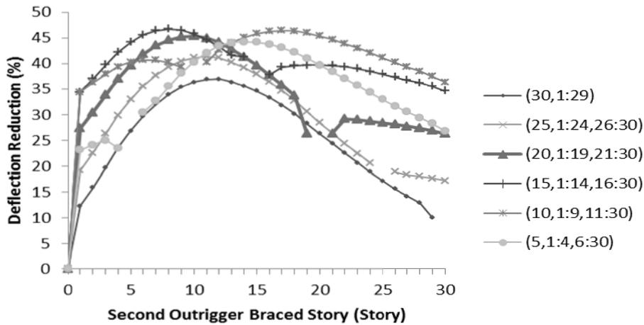
Figure 8. Deflection reduction caused by second outrigger for 30 story model (X-bracing core)
