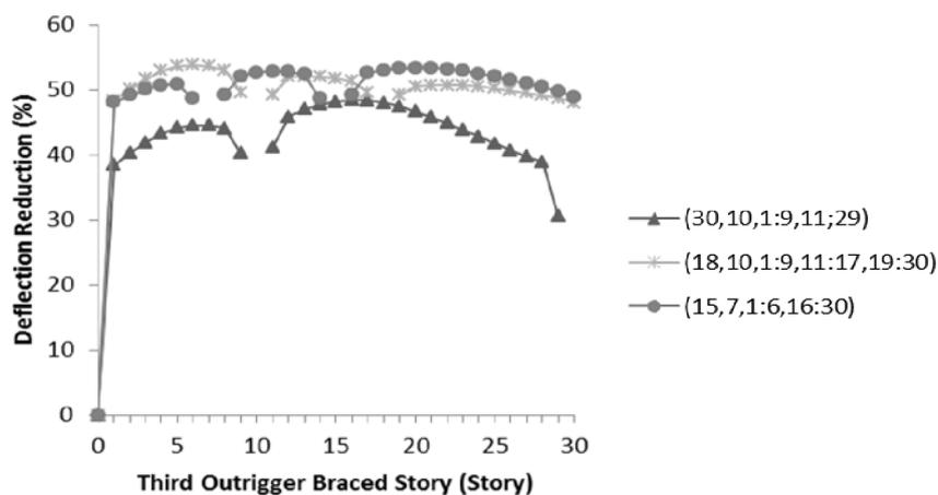
Figure 9. Deflection reduction caused by third outrigger for 30 story model (X-bracing core)
