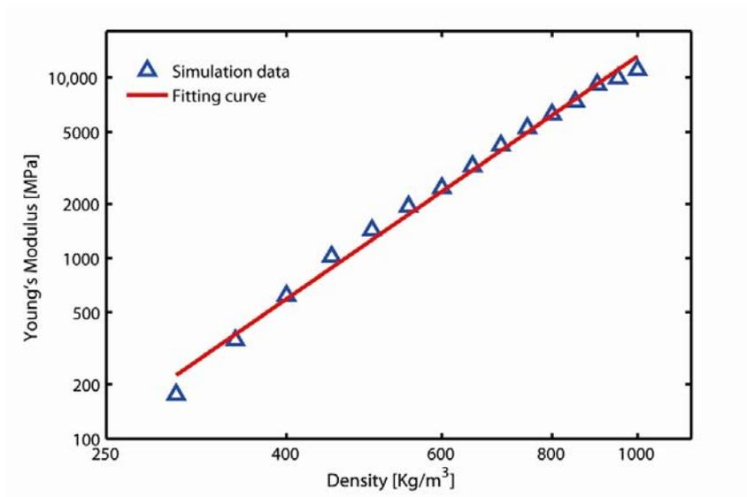
Fig. 2 The relation between Young's modulus and the density in log-log coordinate (The small triangles refer to simulation results. The red curve refers to the power-law fitting curve of simulation data.)
