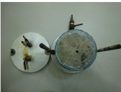
Fig.8 show the edge of sealed single artificial hole of pervious concrete sample before test
