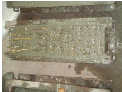
Fig.6 five line of artificial hole of pervious concrete
