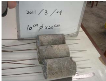
Fig.2 three artificial holes of pervious concrete
