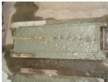
Fig.4 single line of artificial hole of pervious concrete
