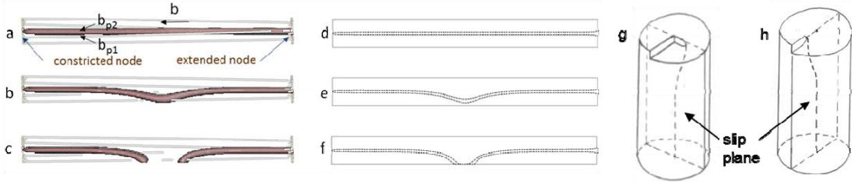
Fig. 1 Atomistic and line tension models of dislocation at metastable state (a,d), activated state (b,e), and escape process (c,f). Diagram for escape from the end, when surface step is nonparallel (g) to the slip plane, and parallel to slip plane (h).
