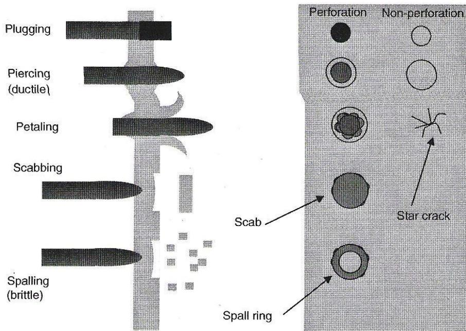
Fig. 3 Target failure modes (Carlucci 2008)
