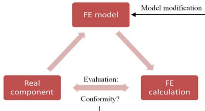
Fig. 2 Basically iterative procedure of an FE analysis
