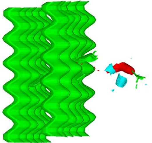
Fig. 14 Numerical simulation of an impact with two corrugated armor plates
