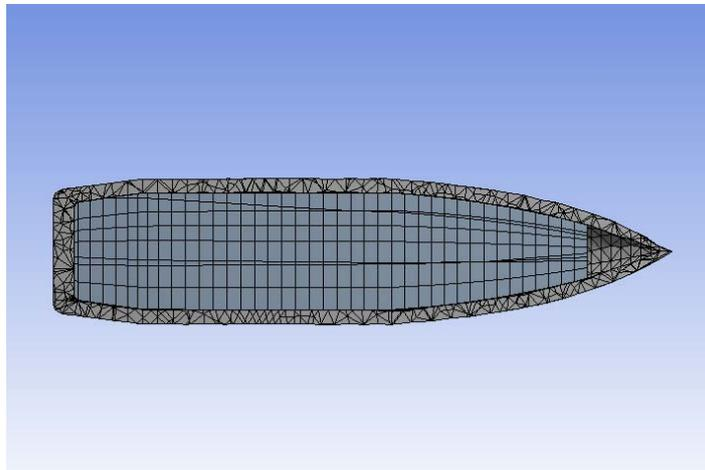
Fig. 7 CAD model of a 7.62 NATO
