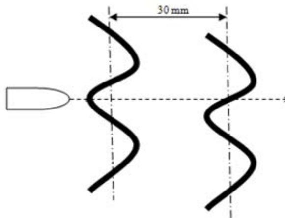
Fig. 13 Modified armor structure with two corrugated plates
