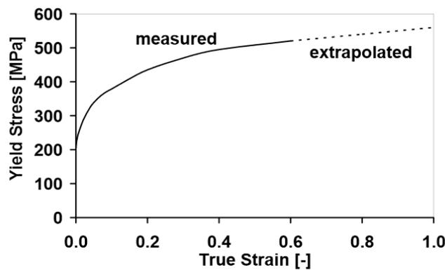
Fig. 8 Extrapolated stress-strain curve
