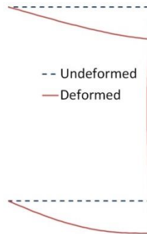
Figure 6 The first buckle mode of the plane frame in Figure 5.
