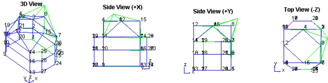
Fig. 4 Mode shape ( $f = 4.029\text{Hz}$ , Amplitude 28%, Phase Angle  $90^\circ$ )
