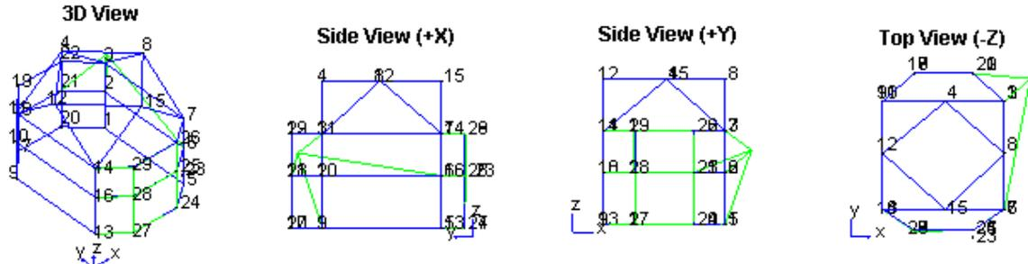
Fig. 5 Mode shape ( $f = 5.392\text{Hz}$ , Amplitude 28%, Phase Angle  $90^\circ$ )
