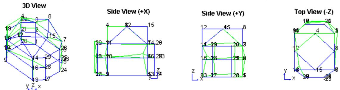
Fig. 6 Mode shape ( $f = 19.91\text{Hz}$ , Amplitude 28%, Phase Angle  $90^\circ$ )
