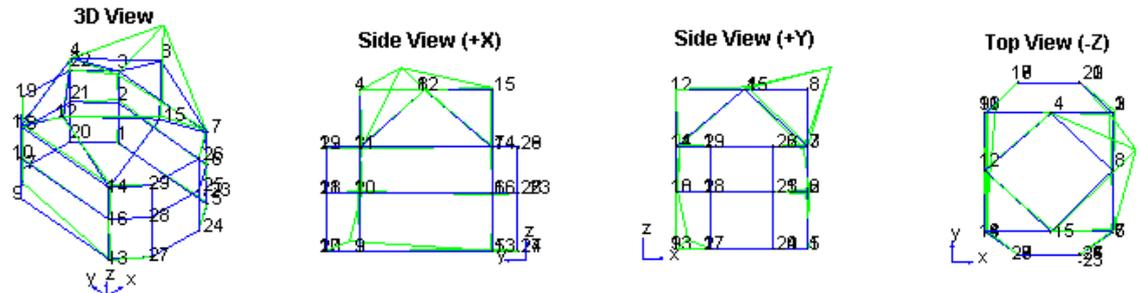
Fig. 3 Mode shape ( $f = 2.115\text{Hz}$ , Amplitude 28%, Phase Angle  $90^\circ$ )
