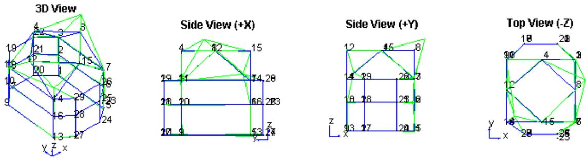
Fig. 2 Mode shape ( $f = 1.722\text{Hz}$ , Amplitude 28%, Phase Angle  $90^\circ$ )
