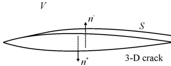
Fig.1 A 3-D crack in an infinite and homogeneous elastic solid  $V$ .
