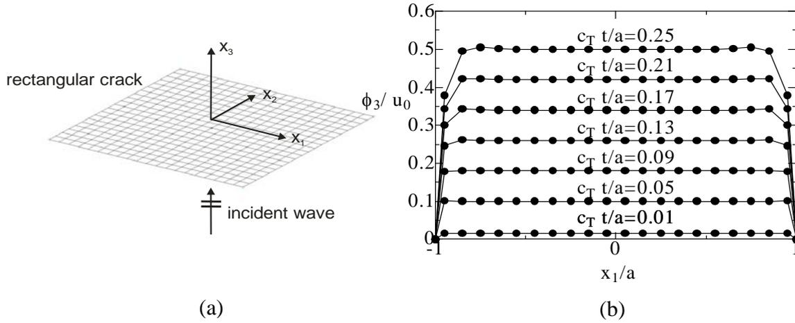
Fig.2 Elastic wave scattering by a rectangular crack. (a) rectangular crack model (b) time variations of crack opening displacements on  $x_1$  axis .
