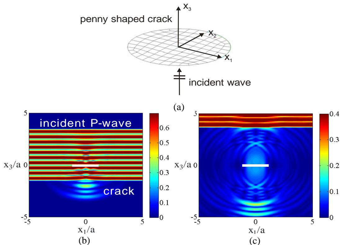
Fig.3 Elastic wave scattering by a penny shaped crack. (a) penny shaped crack model (b) elastic wave field around the crack at  $c_T t/a = 0.5$  (c)  $c_T t/a = 1.9$ .
