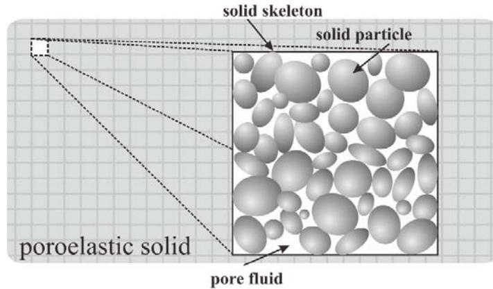
Fig. 1 A schematic of the model of poroelastic solid.
