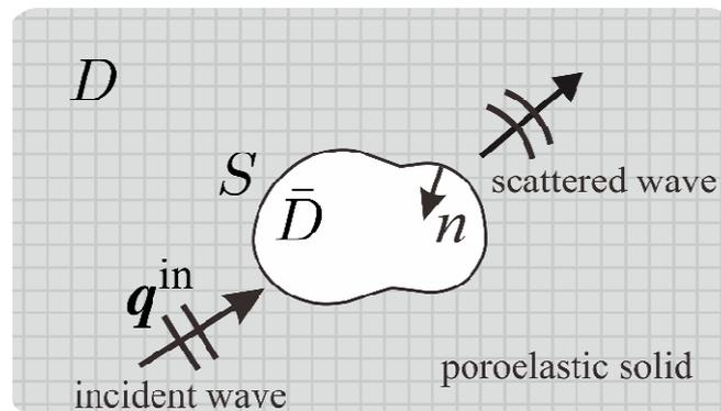
Fig. 2 Wave scattering in a poroelastic medium.
