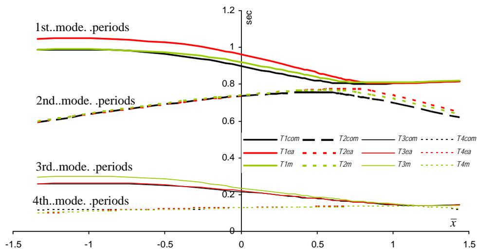
Fig. 5 Periods of vibration of the example structure
