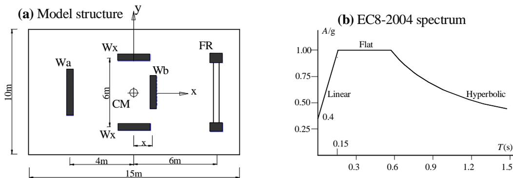
Fig. 4 (a) Floor plan of example structure; (b) Code-recommended design spectrum
