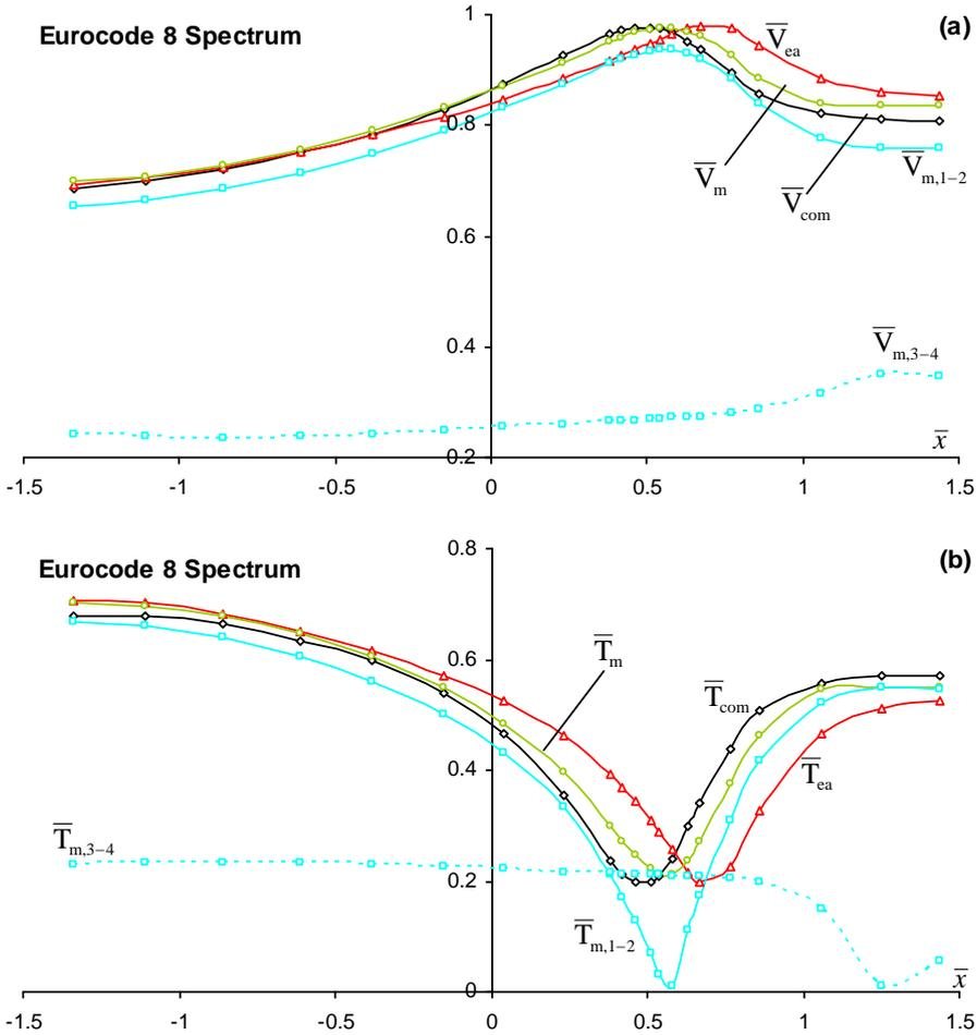
Fig. 7 Peak base shears (a) and torques (b) for the case of EC8-2004 spectrum
