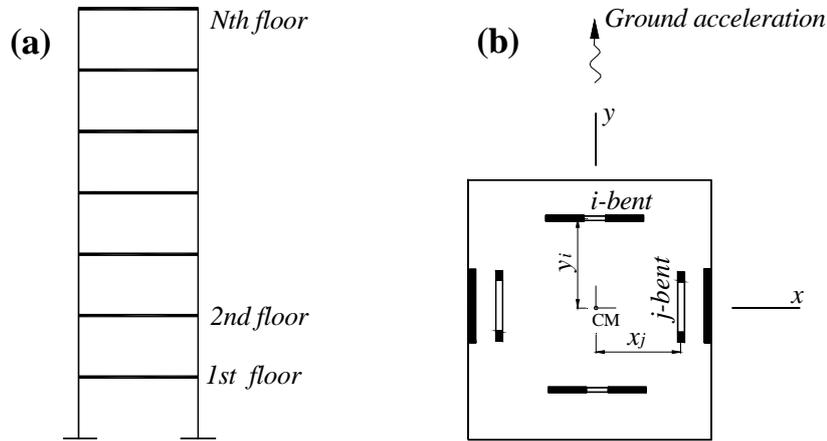
Fig. 1 (a) Elevation of a uniform multi-story building with; (b) symmetrical floor plan
