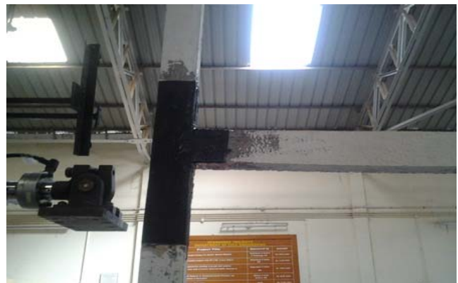
Fig.6(b) Retrofitted Beam-Column joint with carbon fiber reinforced polymer
