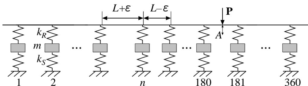
Fig. 3 Track model that  $n$ th sleeper location is shifted
