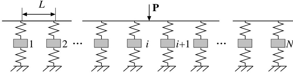
Fig. 2 Track model subjected to a harmonic loading
