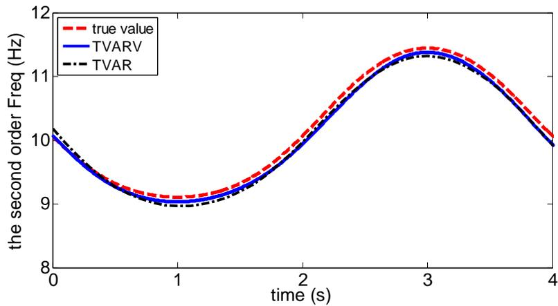
Fig.4 Comparison of 2<sup>nd</sup> instantaneous frequency identified using TVAR and TVARV
