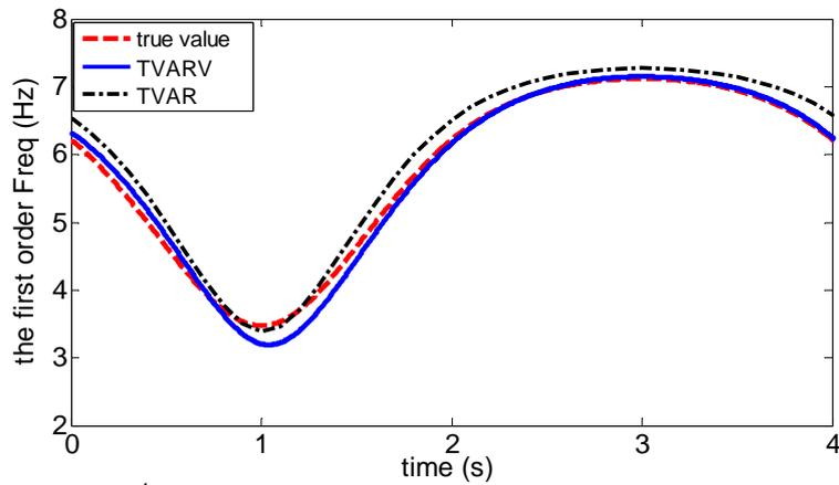
Fig.3 Comparison of 1<sup>st</sup> instantaneous frequency identified using TVAR and TVARV
