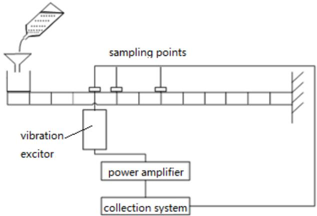
Fig.7 The sketch chart of cantilever beam vibration test
