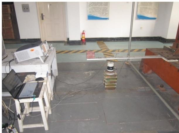
Fig.6 A time-varying cantilever beam test
