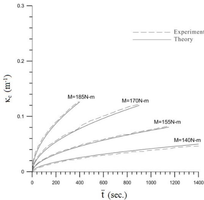
**Fig. 12** The experimental and simulated  $\kappa_c$ - $\bar{t}$  curves for sharp-notched SUS 304 stainless steel tubes with  $a = 0.2$  mm under pure bending creep in the initial and secondary stages
