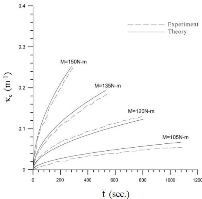
**Fig. 13** The experimental and simulated  $\kappa_c$ - $\bar{t}$  curves for sharp-notched SUS 304 stainless steel tubes with  $a = 0.4$  mm under pure bending creep in the initial and secondary stages
