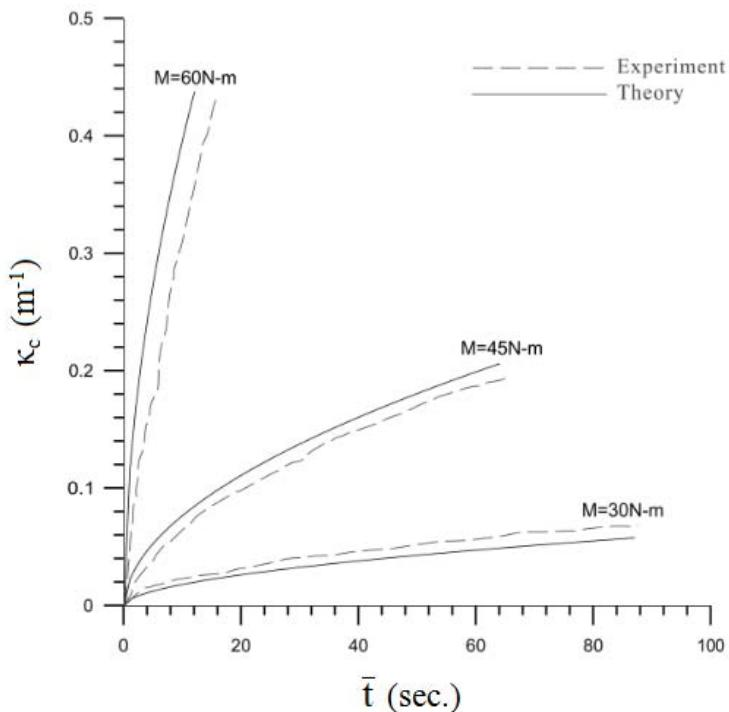
**Fig. 16** The experimental and simulated  $\kappa_c$ - $\bar{t}$  curves for sharp-notched SUS 304 stainless steel tubes with  $a = 1.0$  mm under pure bending creep in the initial and secondary stages
