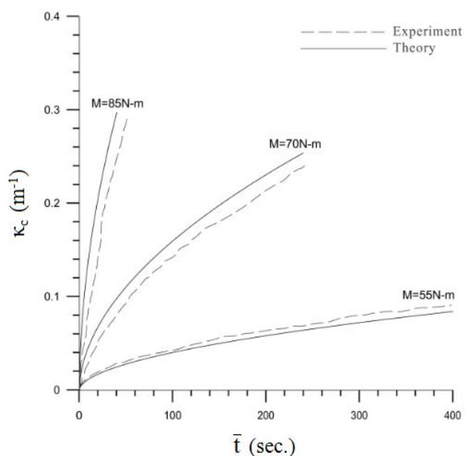
**Fig. 15** The experimental and simulated  $\kappa_c$ - $\bar{t}$  curves for sharp-notched SUS 304 stainless steel tubes with  $a = 0.8$  mm under pure bending creep in the initial and secondary stages
