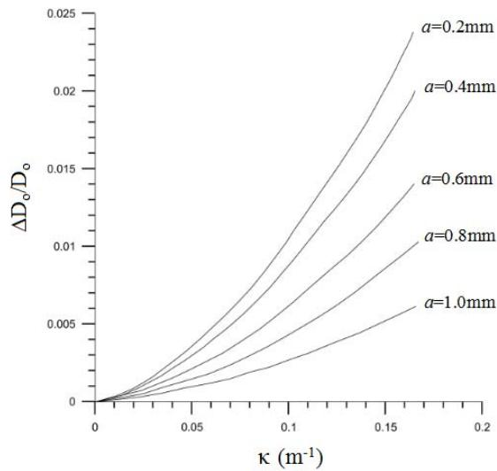
**Fig. 6** The corresponding experimental ovalization ( $\Delta D_0/D_0$ ) - curvature ( $\kappa$ ) curves for sharp-notched SUS 304 stainless steel tubes with different  $a$  under pure bending
