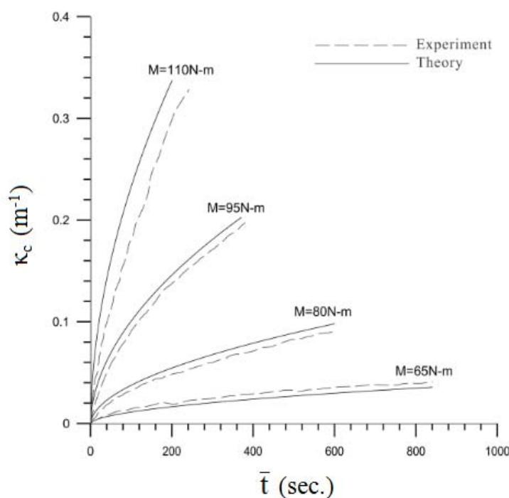
**Fig. 14** The experimental and simulated  $\kappa_c$ - $\bar{t}$  curves for sharp-notched SUS 304 stainless steel tubes with  $a = 0.6$  mm under pure bending creep in the initial and secondary stages
