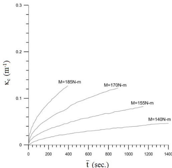
**Fig. 10** The experimental  $\kappa_c$ - $\bar{t}$  curves for sharp-notched SUS 304 stainless steel tubes with  $a = 0.2$  mm under pure bending creep in the initial and secondary stages
