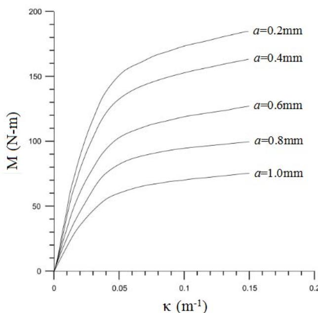
Fig. 5 The experimental moment ( $M$ ) - curvature ( $\kappa$ ) curves for sharp-notched SUS 304 stainless steel tubes with different  $a$  under pure bending
