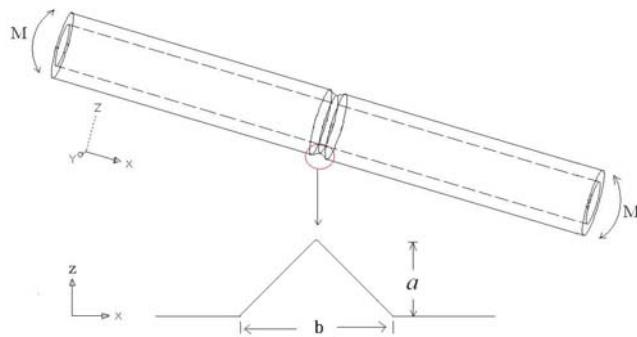
**Fig. 4** A schematic drawing of the sharp-notched tube
