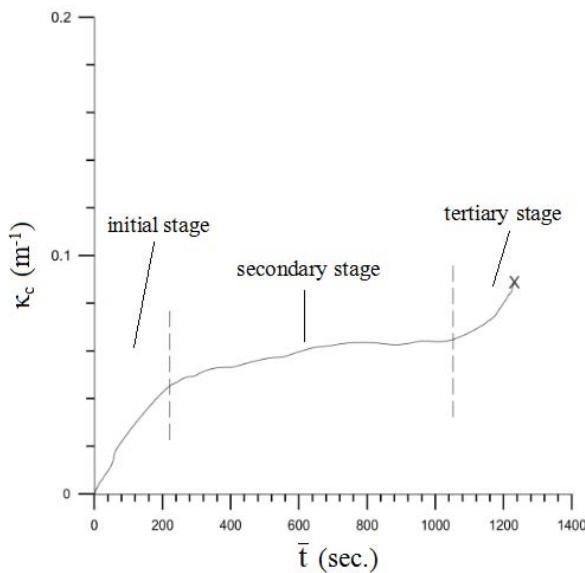
Fig. 8 The creep curvature ( $\kappa_c$ ) – time ( $\bar{t}$ ) curve with the held moment of 155 N-m
