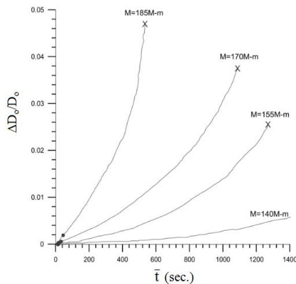
Fig. 9 The corresponding experimental ovalization ( $\Delta D_o/D_o$ ) – time ( $\bar{t}$ ) curves under pure bending and subsequent pure bending creep for Fig. 7
