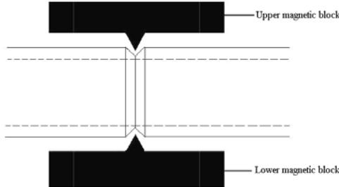
**Fig. 3** Sharp probes on the upper and lower magnetic blocks
