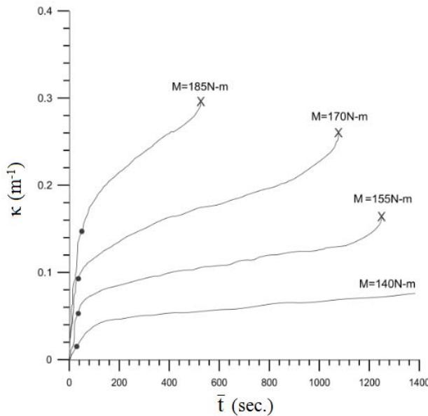
**Fig. 7** The experimental curvature ( $\kappa$ ) – time ( $\bar{t}$ ) curves under pure bending and subsequent pure bending creep for sharp-notched SUS 304 stainless steel tube with  $a = 0.2$  mm
