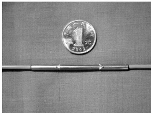
**Fig. 2** Picture of stainless steel tube-packaged FBG strain sensor
