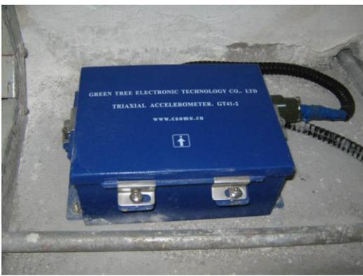
Fig. 7 Accelerometers with steel case
