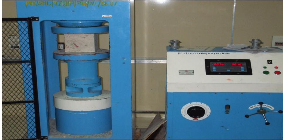
Fig. 3 Compression strength test setup
