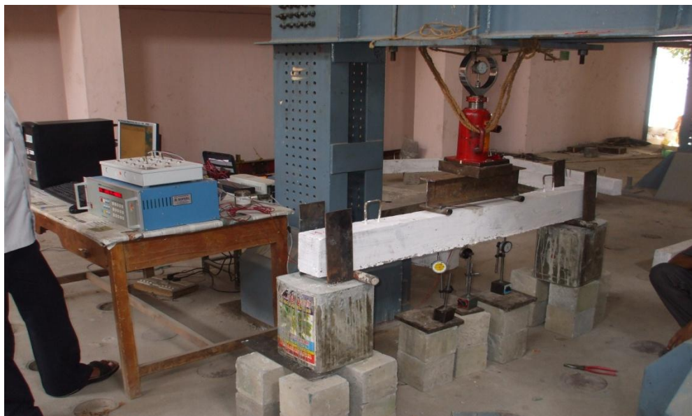
Fig. 4 Flexural strength test setup
