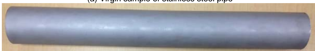
(b) Stainless steel pipe after sand blasting
