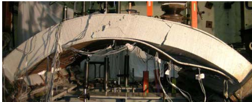
(b) deformed shape of test specimen SA1(Yan, 2012)
