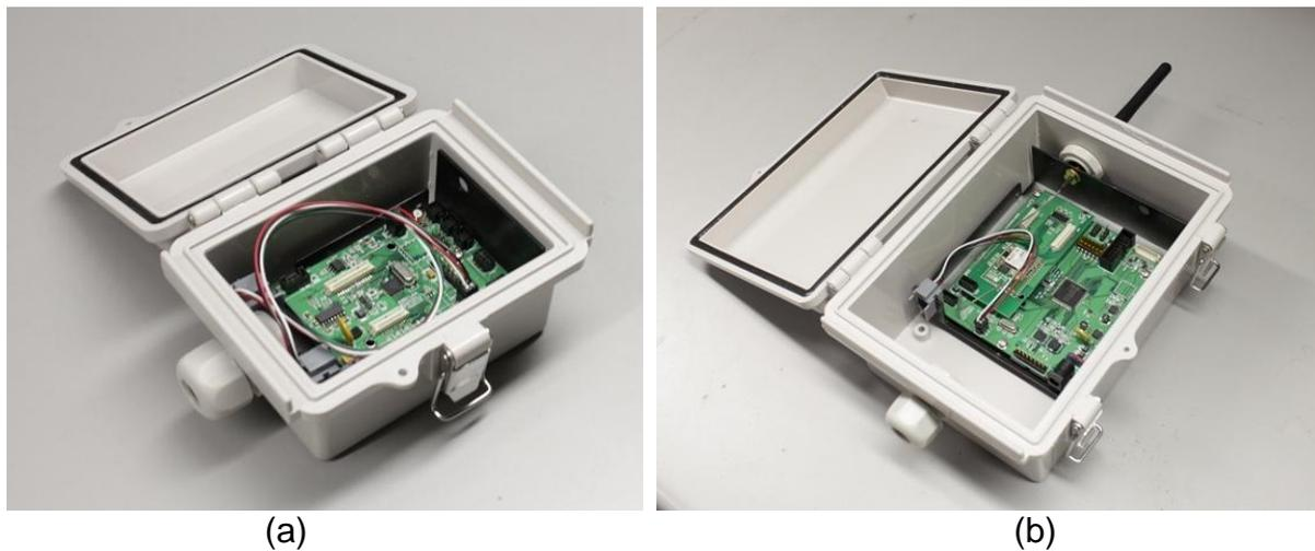
Fig. 3 (a) Sensor node unit, (b) Data aggregator unit
