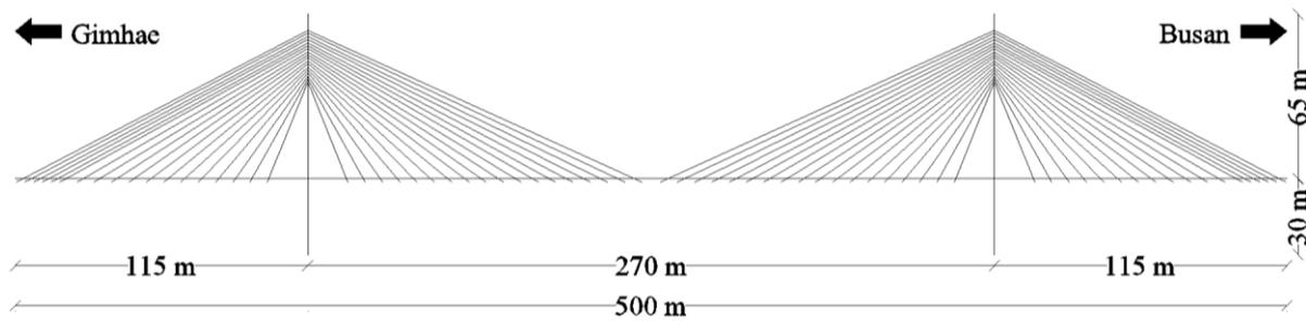
Fig. 2 Layout of the bridge
