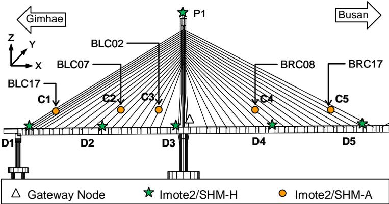
Fig. 7 Imote2 experiment layout (PKNU)
