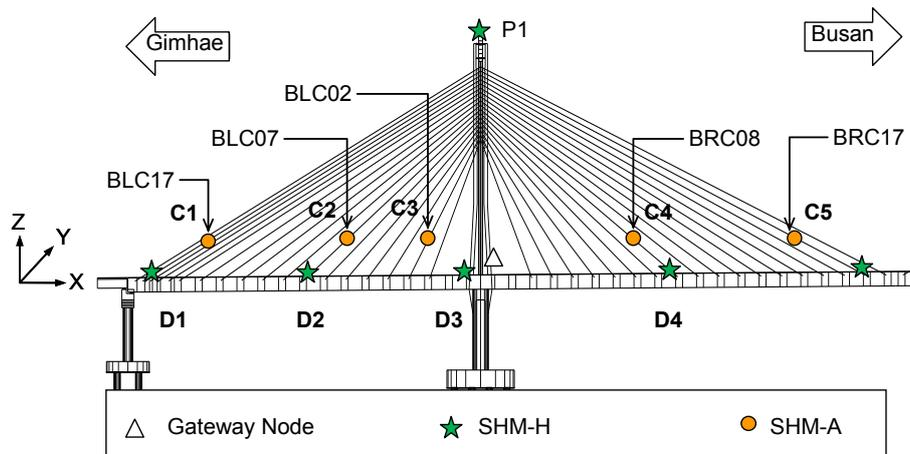
Fig. 4 Sensor layout on the Hwamyung cable-stayed Bridge
