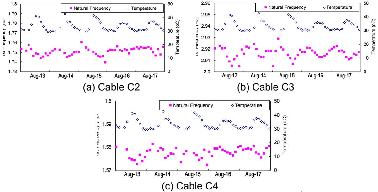
Fig. 9 Monitoring results for short cables C2, C3 and C4 in 5 days: 1<sup>st</sup> natural frequency
