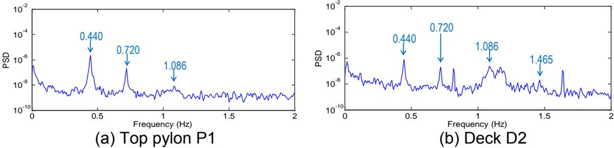
Fig. 6 Frequency responses from sensors on pylon, deck and one cable
