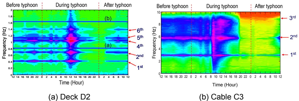
Fig. 13 Time-frequency acceleration response of deck and cable during typhoon Sanba
