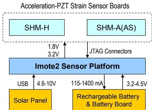
Fig. 2. Schematic of multi-scale sensor node
