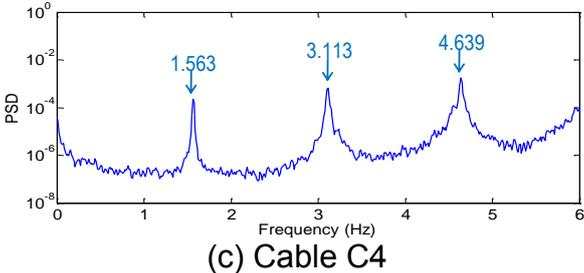
Fig. 6 Frequency responses from sensors on pylon, deck and one cable
