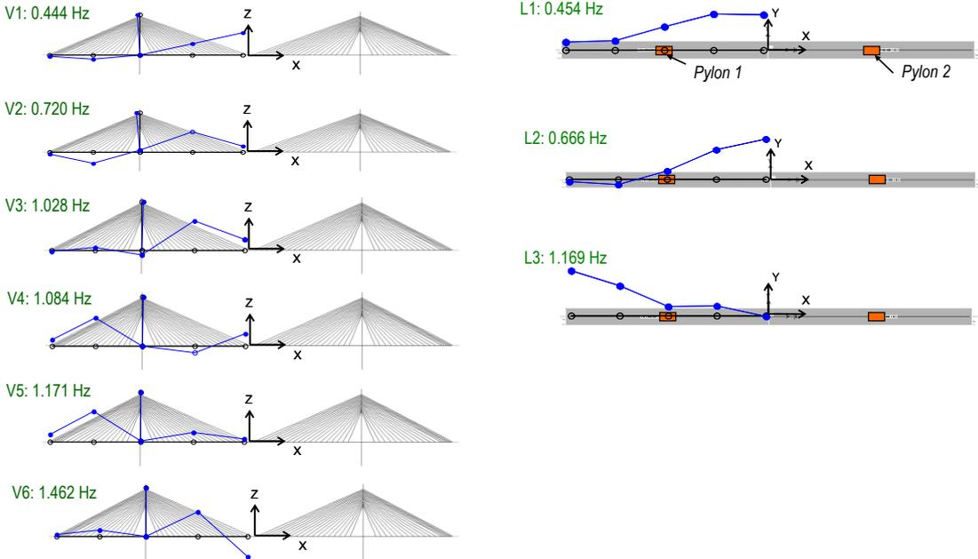
Fig. 7 Identified mode shapes of the Hwamyung Bridge
