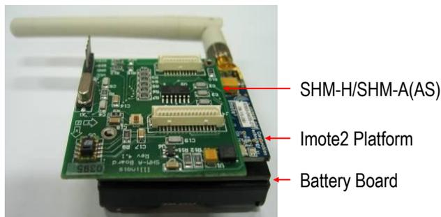
Fig. 3 Prototype of multi-scale sensor node
