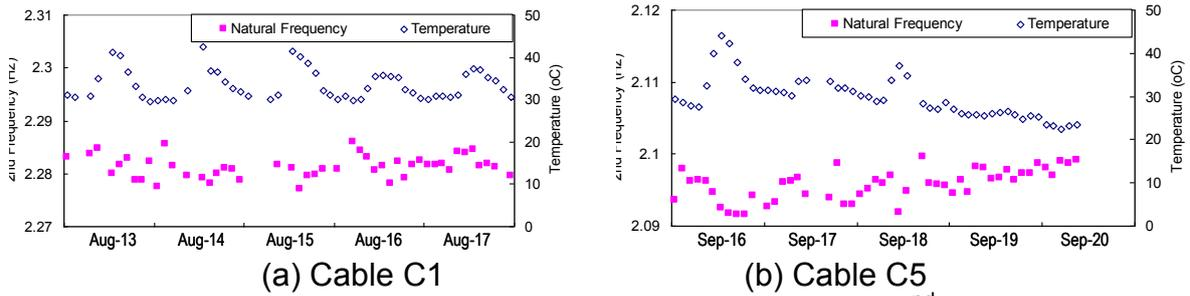
Fig. 10 Monitoring results for long cables C1 and C5 in 5 days: 2<sup>nd</sup> natural frequency
