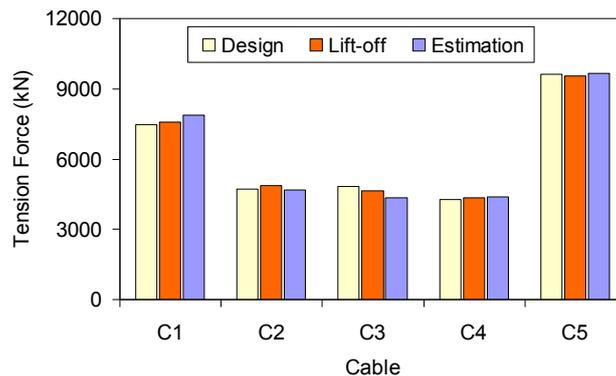
Fig. 8 Cable force estimation: Cables C1-C5
