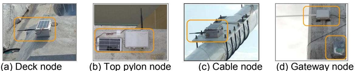
Fig. 5 Field deployment of smart sensor nodes on Hwamyung Bridge
