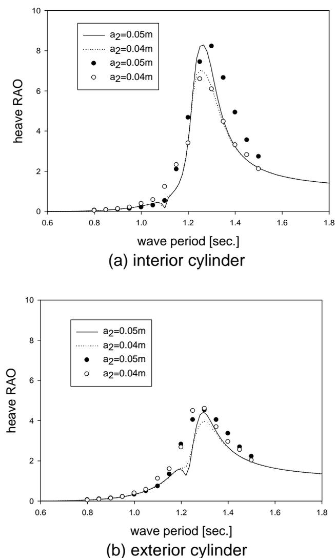
**Fig. 3** Comparison between the analytic solutions and experimental results as function of the inner radius of the exterior cylinder and wave period (lines: analytic solution, symbols: experimental result) for  $a_1 = 0.037m$ ,  $a_3 = 0.1m$ ,  $d_1 = 0.35m$ ,  $d_2 = 0.29m$ .
