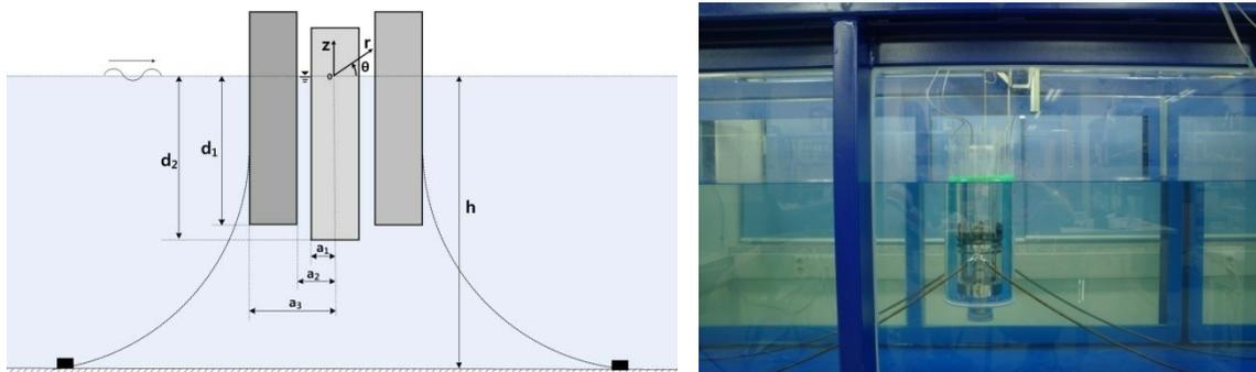
**Fig.1** Schematic representation and experimental model of two concentric cylinders.
