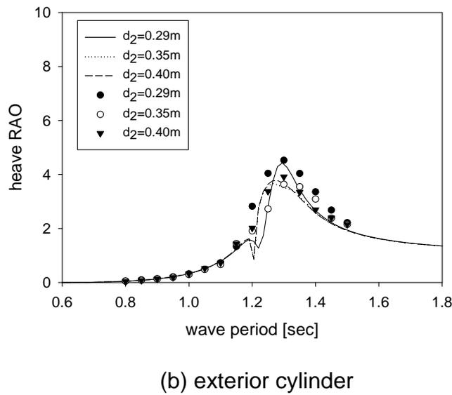
**Fig. 2** Comparison between the analytic solutions and experimental results as function of the draft of interior cylinder and wave period (lines: analytic solution, symbols: experimental result) for  $a_1 = 0.037\text{m}$ ,  $a_2 = 0.05\text{m}$ ,  $a_3 = 0.1\text{m}$ , and  $d_1 = 0.35\text{m}$ .
