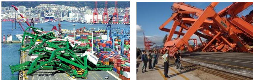
Fig. 1 Crane collapse by Typhoon in Pusan ports (Gamman, Jasungdae, 2003)
