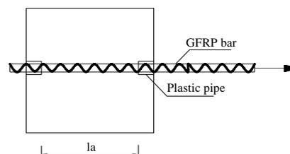
Fig. 2 Standard test block schematic diagram
