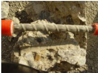
Fig. 5 The intercostal concrete splitting failure
