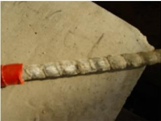
Fig. 4 The ribs stripping GFRP bars
