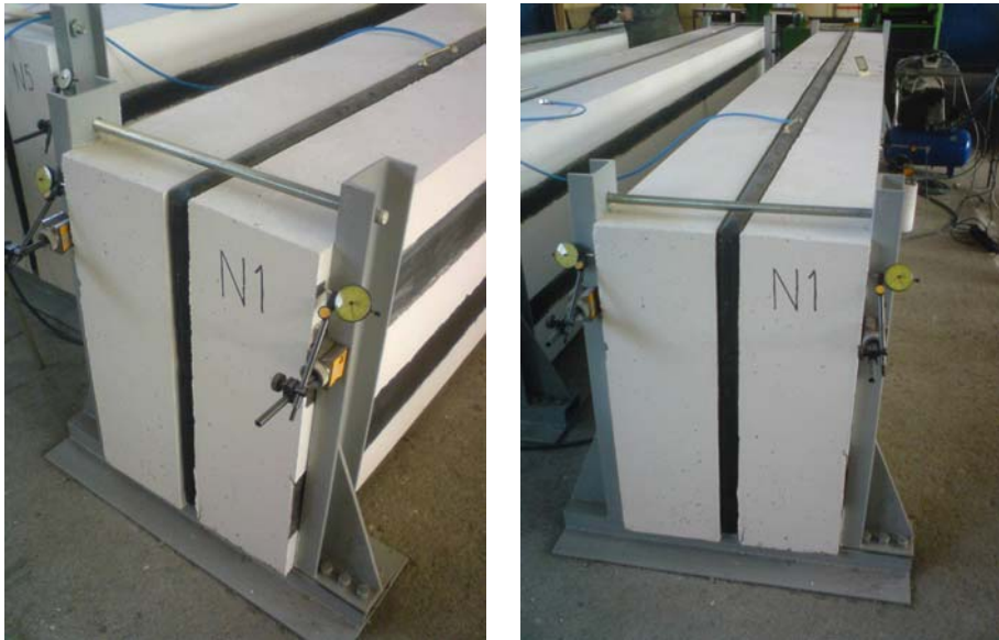
Figure 6: Loaded beams in the steel frame
