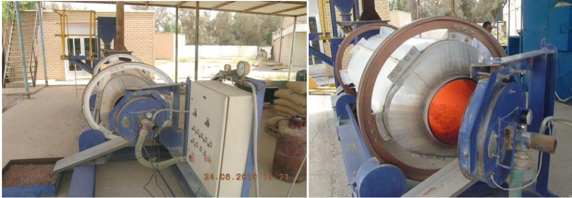
Figure 5. Pilot rotary trefoil kiln.
