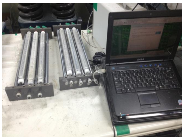
Fig 5 Test specimens of corrugated PE molds after the experiments
