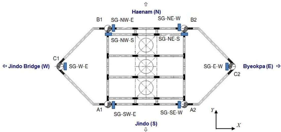
Fig. 3 Installation Locations of Strain Gauges
