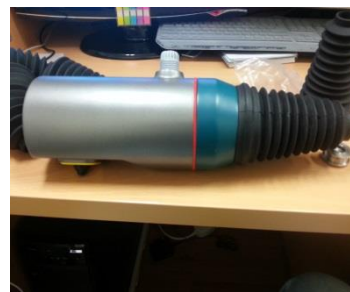
Fig. 2 Schmidt hammer after waterproof
