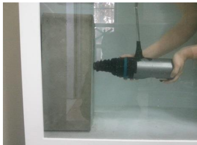
Fig. 6 Rebound Hardness Test in under water condition
