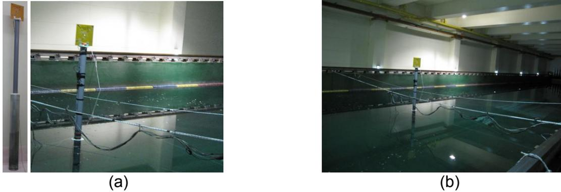
Fig. 4. Experimental setup for obtaining the dynamic response of the moored scale model: (a) scale model (b) one-directional wave tank.
