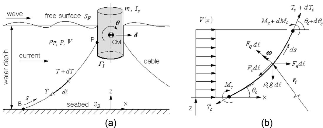
Fig. 2 (a) A rigid floating body moored by catenary cables in irregular wave (b) forces acting on the cable element.
