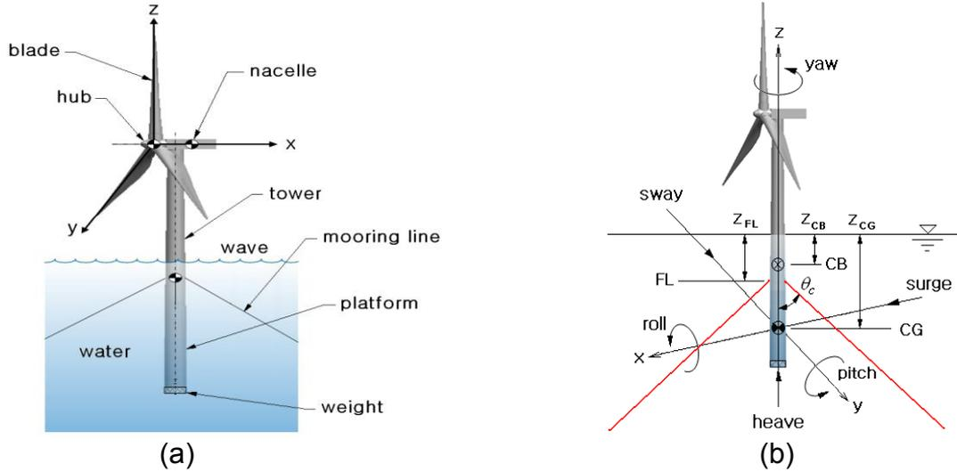
Fig. 1 (a) Spar-type floating offshore wind turbine, (b) 6-DOF rigid body motions.
