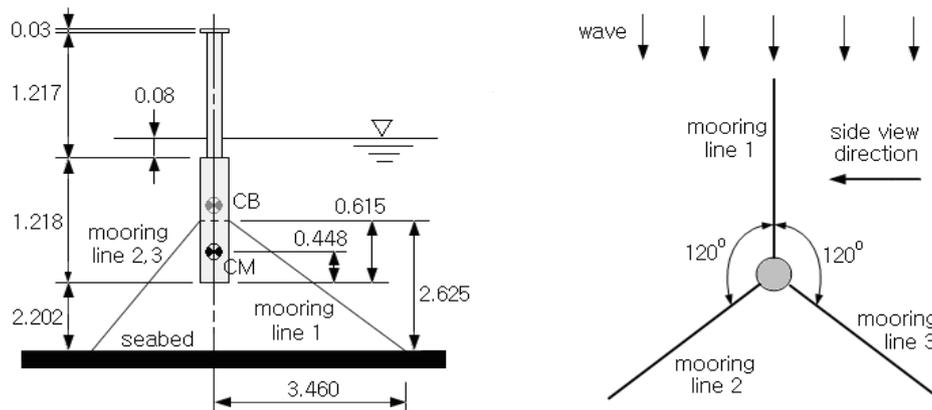
Fig. 3 A simplified spar-type platform moored by three nylon cables (unit:  $m$ )
