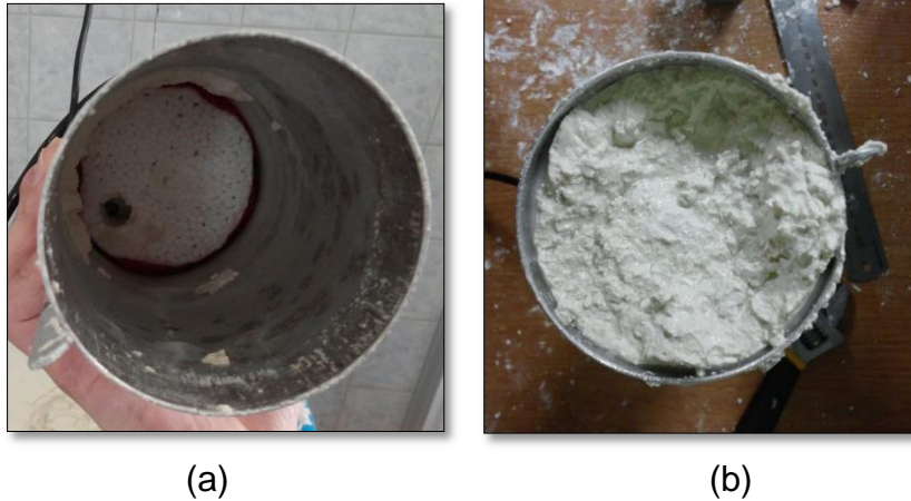
Fig. 8 Failures with soil (a) unplugged and (b) plugged
