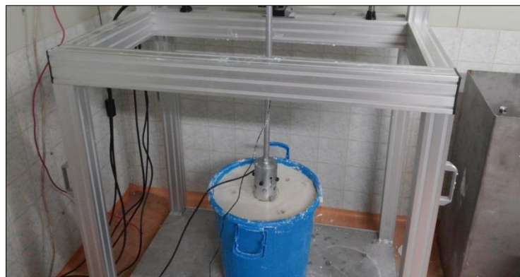
Fig. 3 Experimental set-up of suction anchor static pull-out
