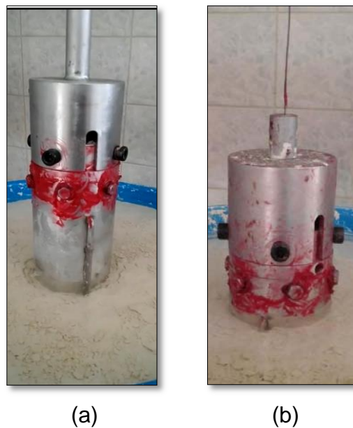
Fig. 5 Model caisson set for (a) installation and (b) pullout
