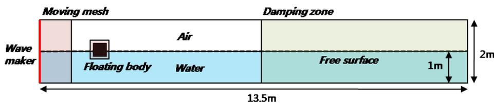
Fig. 6 Schematic view of the entire computation domain for a flume with a floating body
