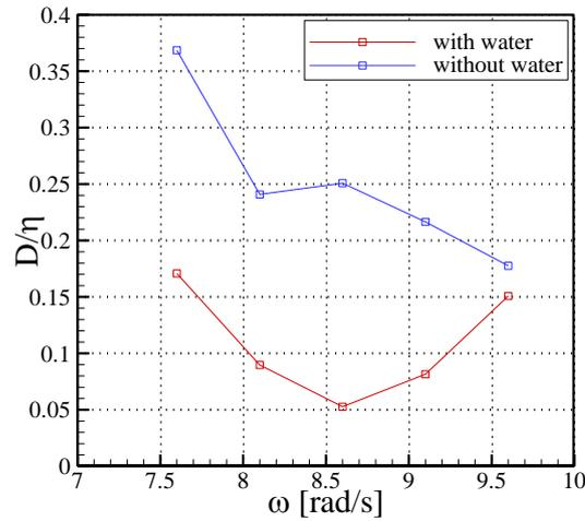
Fig. 7 Non-dimensional amplitudes of surge motion of a floating body with and without water
