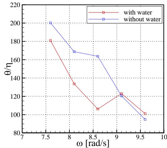
Fig. 8 Non-dimensional pitch motion of a floating body with and without water
