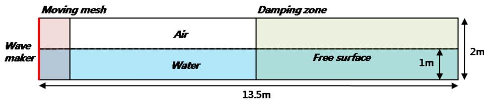
Fig. 3 Schematic view of the entire computation domain for a flume
