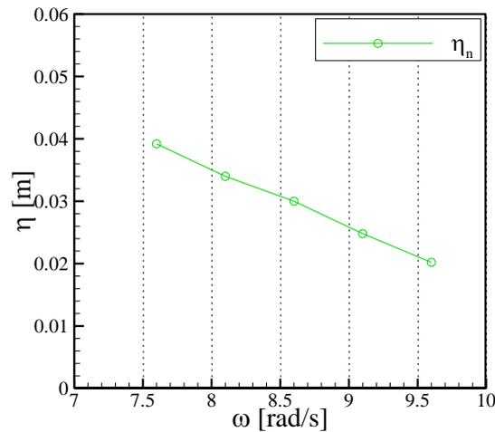
Fig. 5 Variation of amplitude of surface wave according to the excitation frequency
