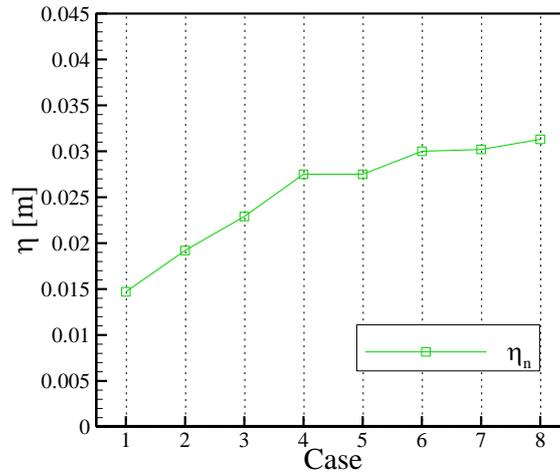
Fig. 4 Predicted amplitude of surface wave according to grid resolution (The higher case number means the simulation result using denser grids)
