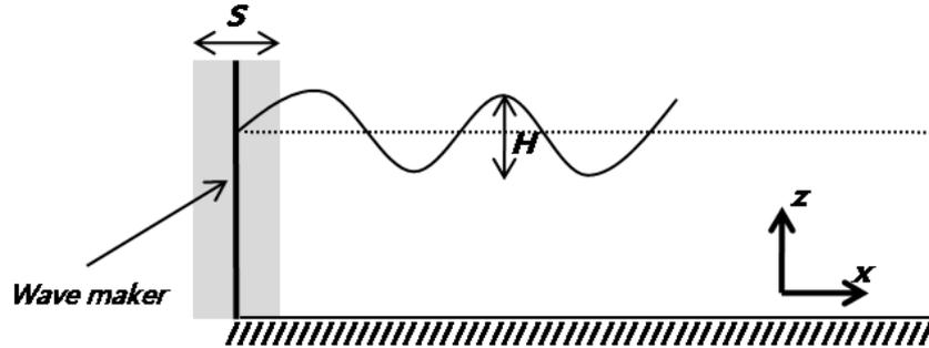
Fig. 2 A wave maker and surface wave
