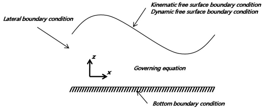
Fig. 1 Boundary conditions for deriving potential theory of surface wave
