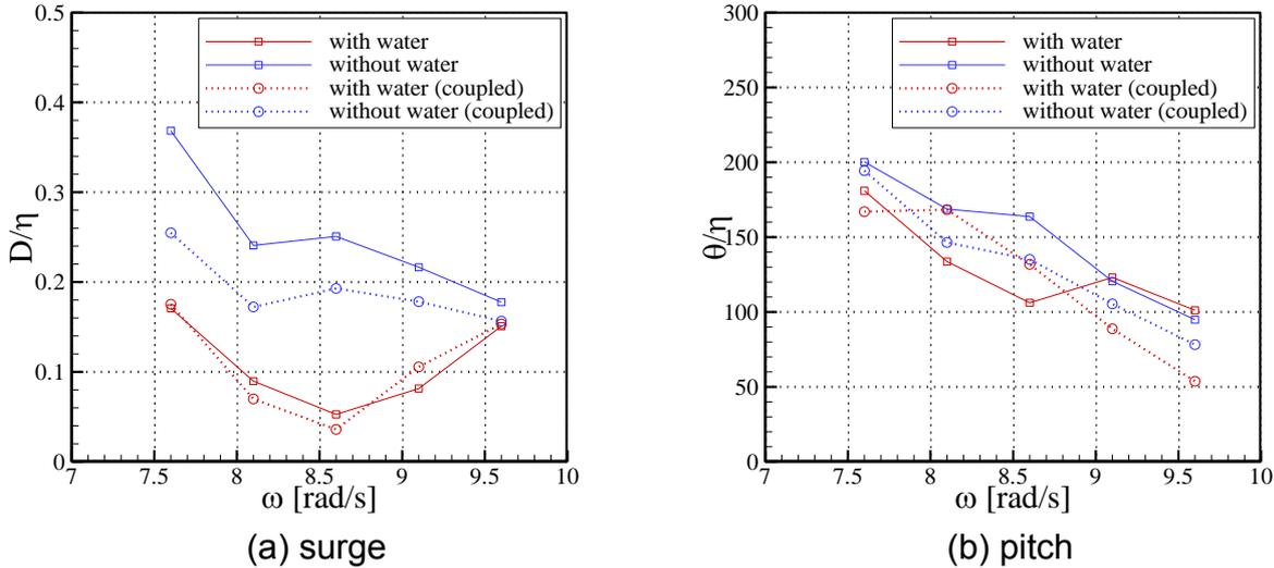
Fig. 9 Non-dimensional coupled surge and pitch motions of a floating body with and without water
