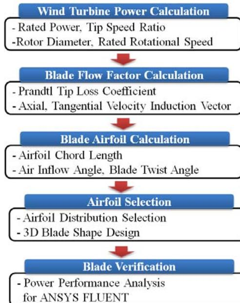
Fig. 2. Design Flow Chart of Wind Turbine Blade
