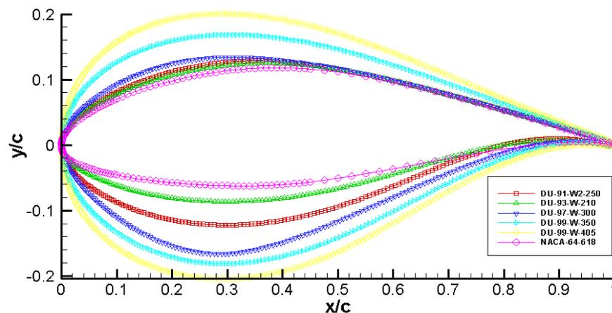
Fig. 1. Airfoil Shape of Wind Turbine Blade
