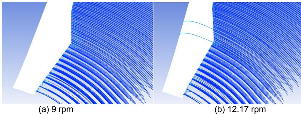
Fig. 8. Streamlines of Pressure Distribution at Blade Root Region
