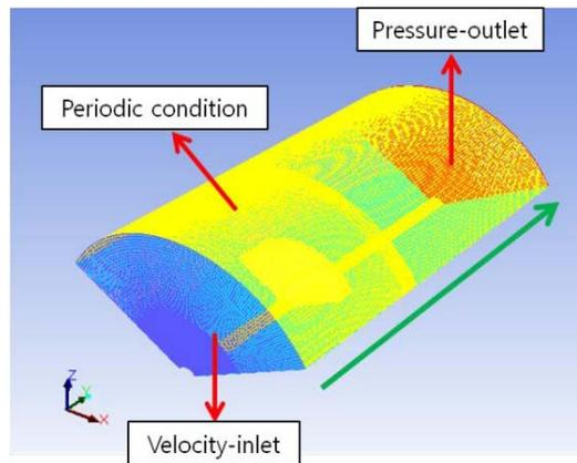
Fig. 6. Computational Domain and Boundary Condition
