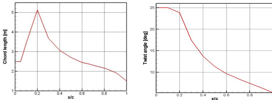
Fig. 3. Chord Length and Twist Angle v/s x/c
