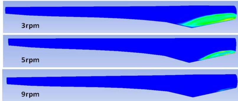
Fig. 10. Turbulence Viscosity Distribution with Change in Rotational Speed
