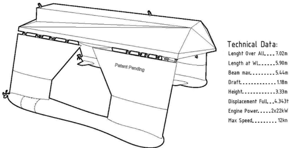
Figure 1- USV-SWATH for Launching, Recovering and Recharging of AUVs
