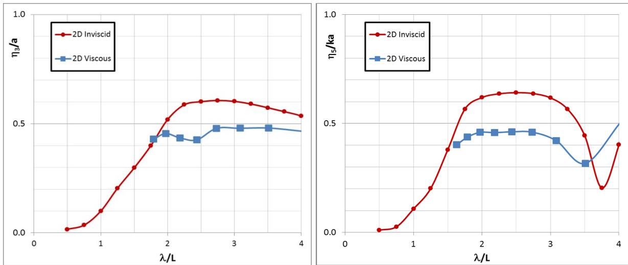
Figure 7 – Response Amplitude Operators of Heave ( $\eta_3$ ) and Pitch ( $\eta_5$ )
