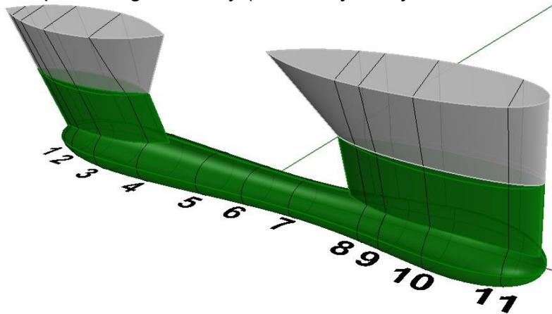
Figure 3 – Geometry of a SWATH demi-hull with position of the 11 sections considered to calculate the viscous added mass and damping
