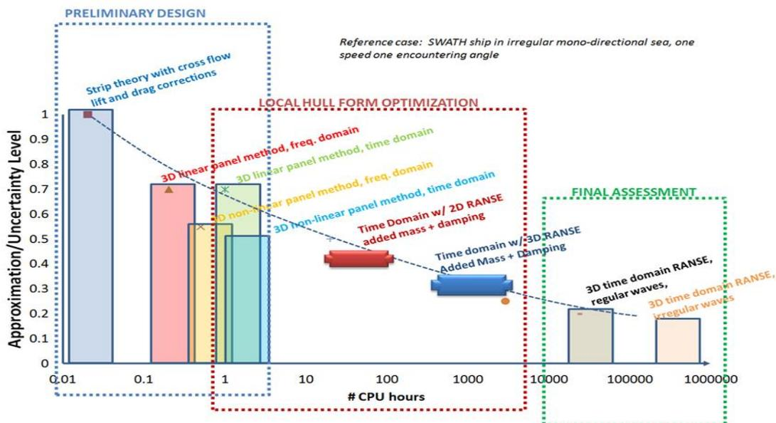
Figure 2 – Accuracy vs. computational time of different numerical methods for the motion prediction of SWATH ship in waves. Considered methods range from 2D potential flow theories to unsteady 3D viscous flow solvers.
