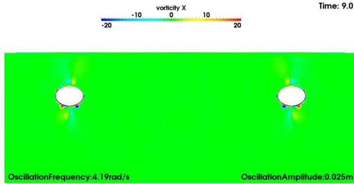
Figure 4 – Snapshot of the predicted viscous flow field (vorticity) for station 1, 4 and 6 respectively for the heave radiation problem.
