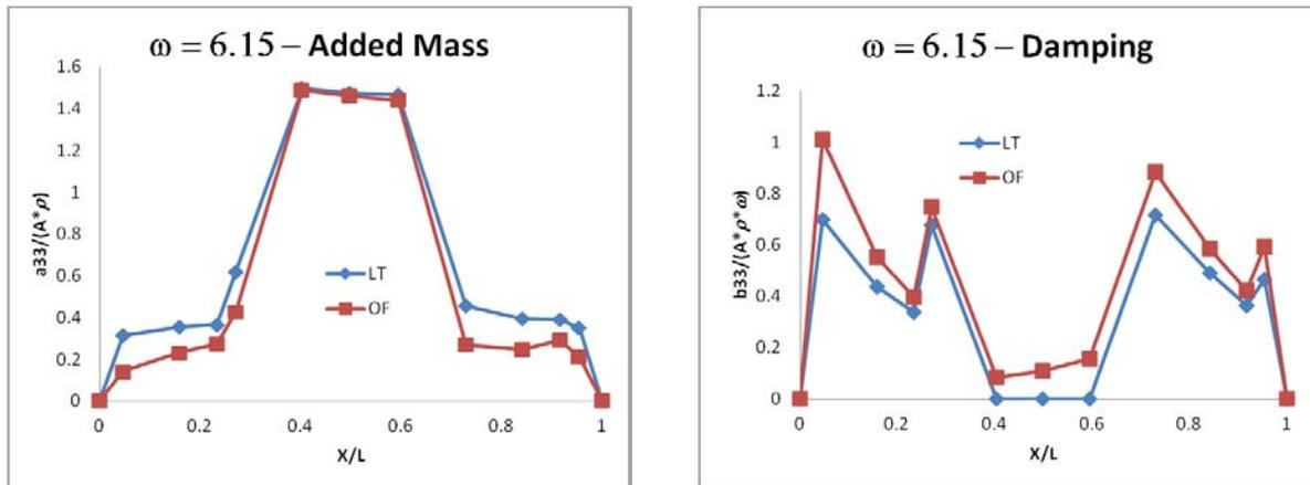
Figure 5 - Sectional heave added mass ( $a_{33}$ ) and damping ( $b_{33}$ ) calculated with inviscid (LT) and viscous (OF) methods at three different oscillation frequencies plot along ship length.
