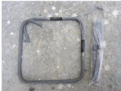
Fig. 5 Transverse reinforcement with strain gauges
