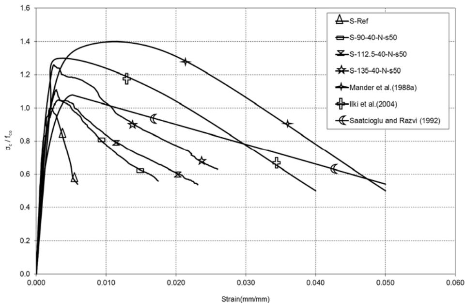
Fig. 9 Predicted stress-strain relationships for the first group specimens
