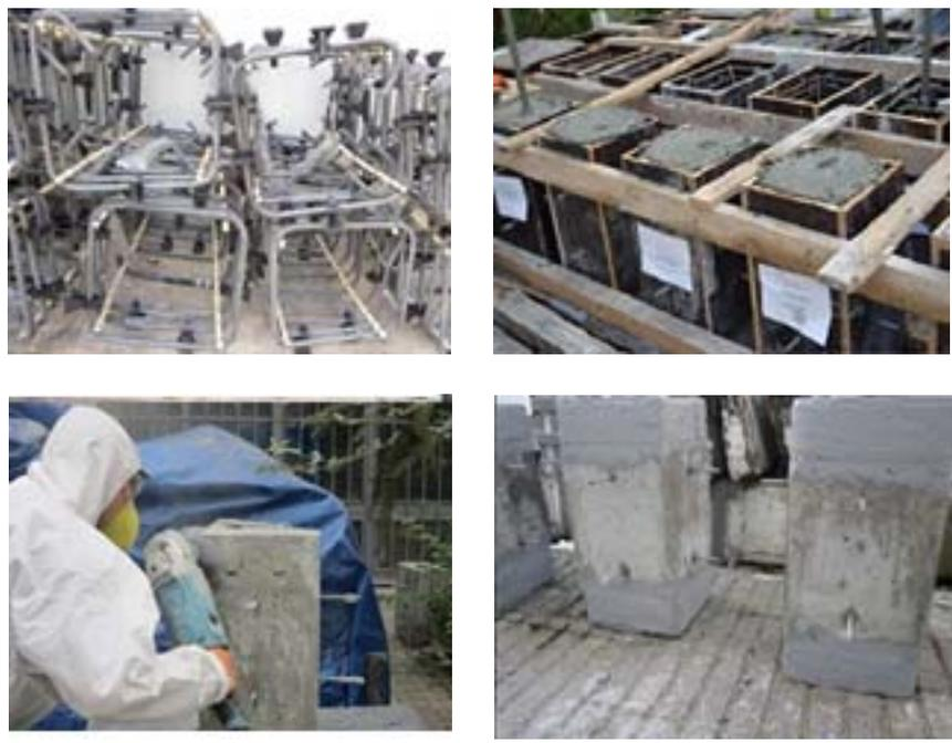
Fig. 3 Specimen preparation
