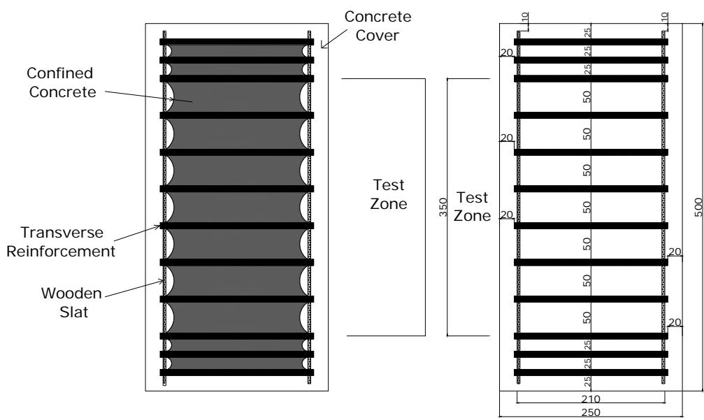
Fig. 2 Transverse reinforcement detailing (all dimensions are in mm)
