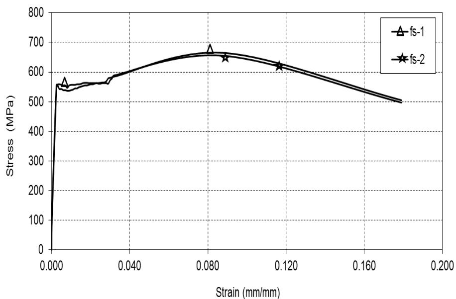
Fig. 1 Stress-strain relationships of transverse reinforcement
