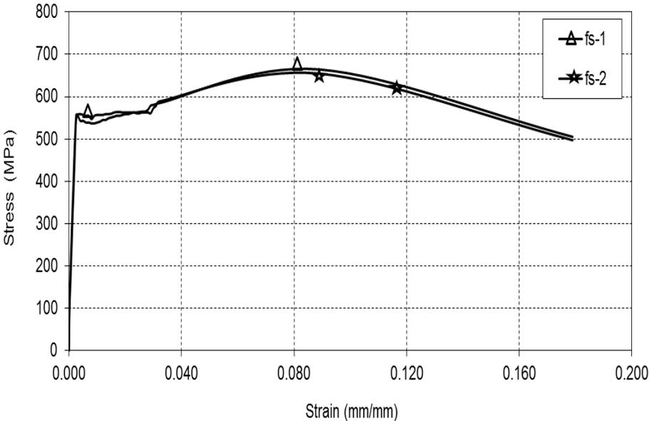
Fig. 1 Stress-strain relationships of transverse reinforcement
