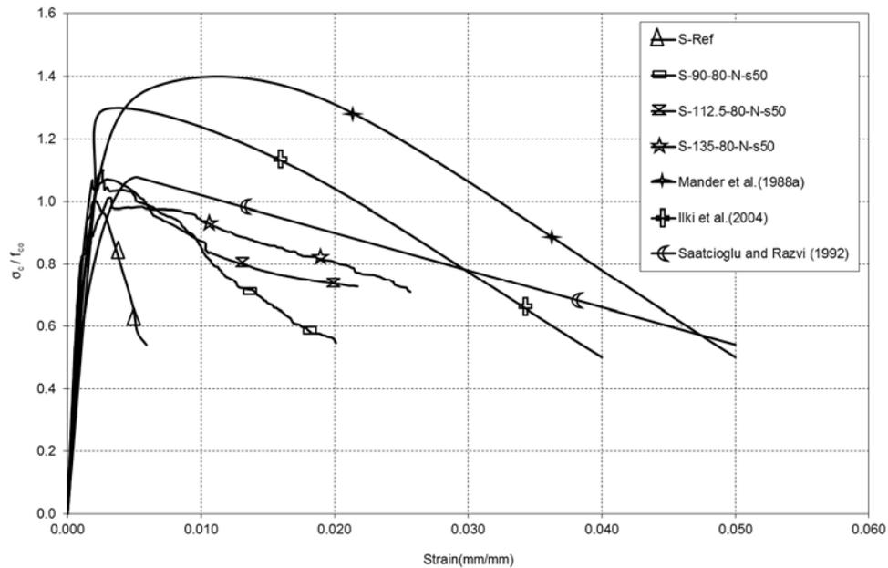
Fig. 10 Predicted stress-strain relationships for the second group specimens
