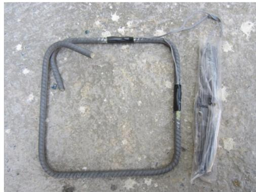
Fig. 5 Transverse reinforcement with strain gauges
