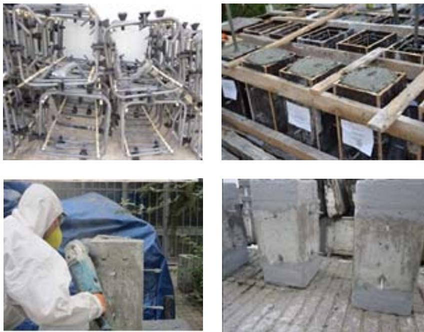
Fig. 3 Specimen preparation
