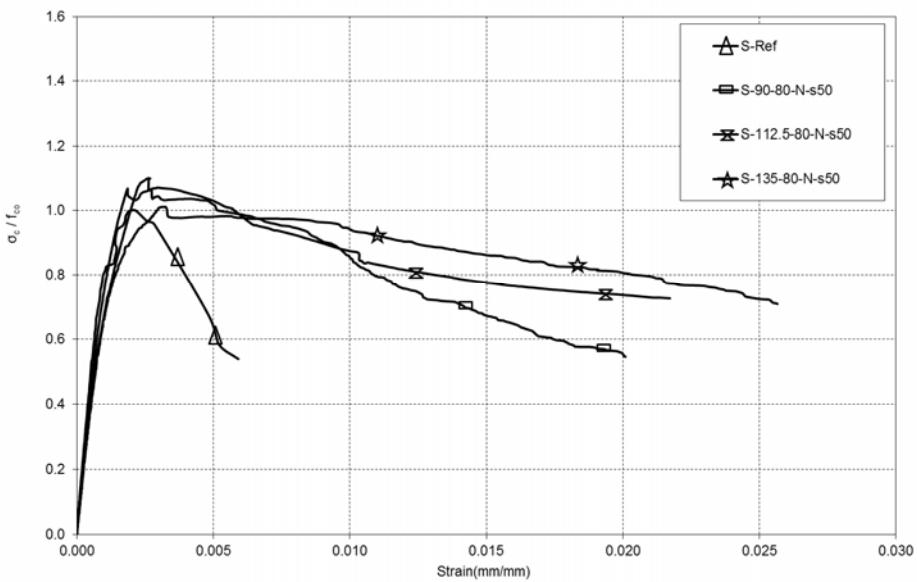
Fig. 7 Stress – strain relationships of the second group specimens
