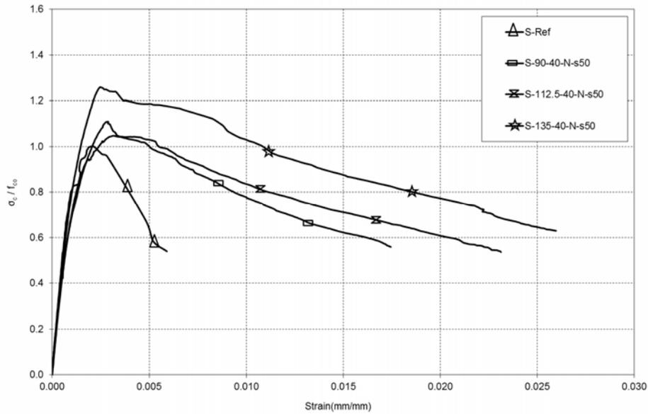
Fig. 6 Stress – strain relationships of the first group specimens
