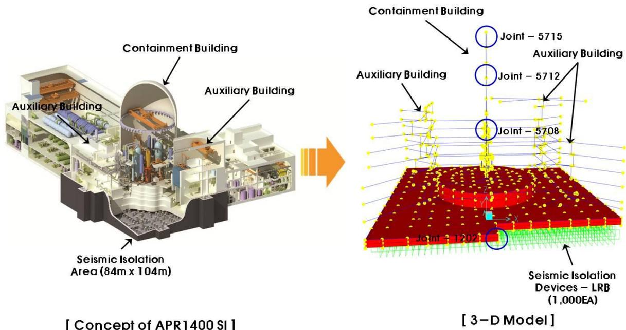
Fig. 3 Concept diagram of NPP seismic isolation system and 3-dimensional analysis model
