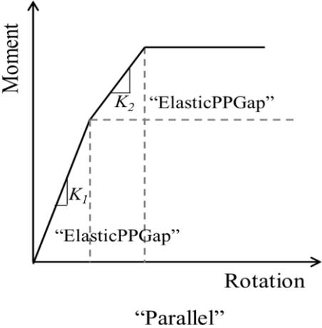
Fig. 3 Multi-Linear Model for Monotonic Loading (Mazzoni and et al., 2006)
