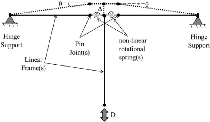
Fig. 2 The FE Model of T-joint System
