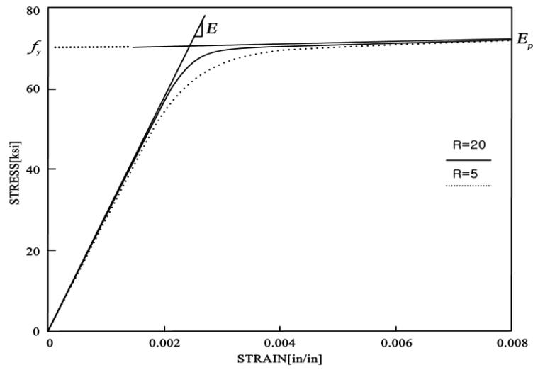
Fig. 5 Steel02 Material in OpenSees (Mazzoni and et al., 2006)
