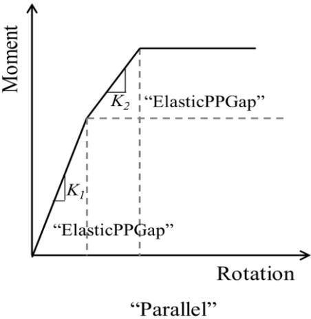
Fig. 3 Multi-Linear Model for Monotonic Loading (Mazzoni and et al., 2006)
