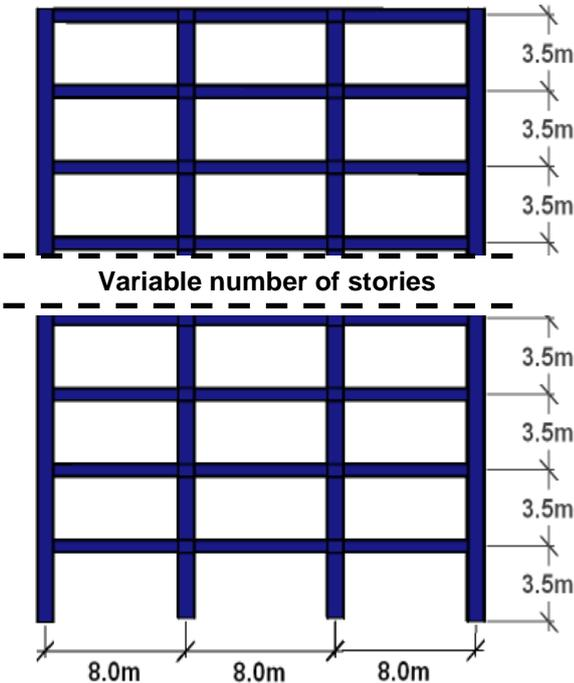
Fig. 1 Geometrical characteristics of the steel frames
