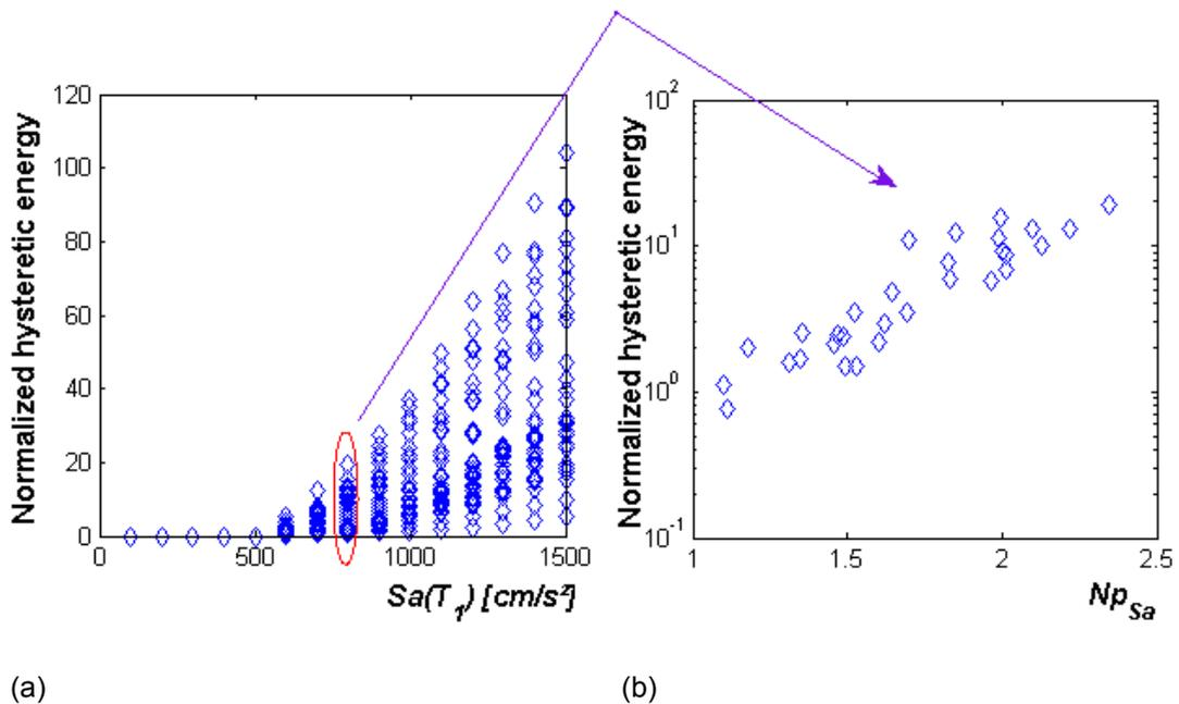
Fig. 2 (a) Incremental dynamic analysis scaling for  $Sa(T_1)$ ; (b) Relation between  $N_{pSa}$  and the normalized hysteretic energy at  $Sa(T_1)=800\text{cm/s}^2$
